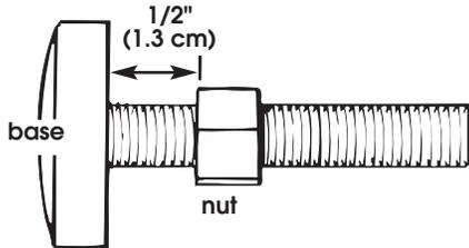
**10.** Use legs and nuts from parts package. Screw nut down to within 1/2 inch (1.3 cm) of base.
