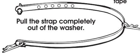
**1.** Remove tape that covers shipping strap. Pull to completely remove the shipping strap with 2 cotterpins from the inside of the washer.
