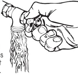
**8.** Attach bottom hose (inlet marked "H") to hot water faucet. Attach top hose (inlet marked "C") to cold water faucet. Tighten coupling to faucet by hand; then use pliers to make final two-thirds turn.
