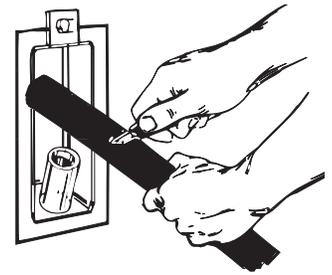
**4.** Move washer close to final position. Put "hook" end of drain hose into standpipe. Estimate length of drain hose needed when washer is in final position. Hose must be cut exactly to length so "hook" end is held tightly over edge of standpipe. If drain hose is too long, cut straight end of hose. (Do Not cut "hook" shaped end of drain hose.)
