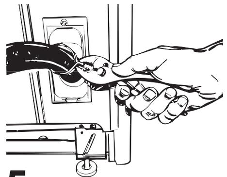
**5.** Place hose clamp over washer drain connector. Push drain hose onto washer connector. Use pliers to open clamp and slide clamp over drain hose. Check for good fit.
