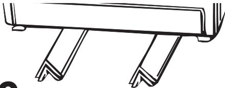
**9.** Stack two corner posts on top of each other. Tilt washer backwards and insert corner posts 3 inches (7.6 cm) in from one side of washer as shown. Repeat with other corner posts on other side of washer.
