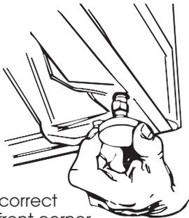
**11.** Insert legs into correct holes at each front corner of washer until nuts touch washer. **Do Not** tighten nuts until Step 14.
