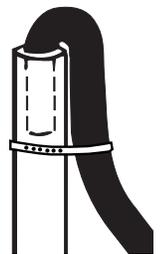
**7.** Before attaching water inlet hoses, run water through both faucets into a bucket. This will get rid of particles in water lines that might clog hoses. Mark which is the hot water faucet.
