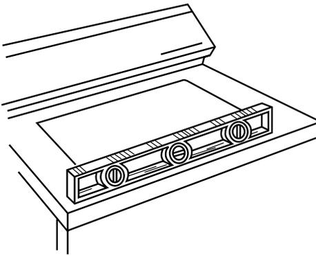
**13.** Tilt washer forward raising back legs 1 inch (2.5 cm) off of floor. To adjust rear self-leveling legs, gently lower washer to floor. Check levelness of the washer by placing a carpenter's level on top of the washer, first side to side; then front to back.
