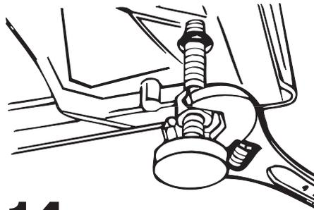
**14.** If washer is not level, adjust the front legs up or down. Make final check with level.
