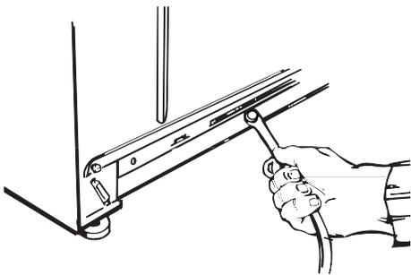
Pull firmly to remove the end of shipping strap from the back of the washer. The shipping strap plug must be completely removed from the washer for the self-leveling legs to be released.
