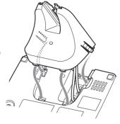
For a wall plate, align the base's keyhole slots with the wall plate studs and slide the base downward to secure it.
