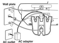
For direct wall mounting, route the telephone cord through the bracket's groove. Then align the base's keyhole slots with the mounting screws and slide the base downward to secure it.
