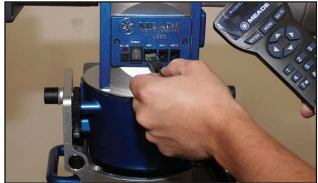
Fig 24: Plug AudioStar into HBX connector
