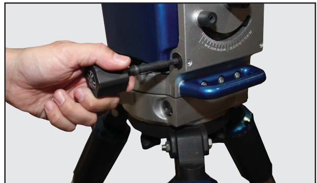
Fig 27: Removing the hex head tool
