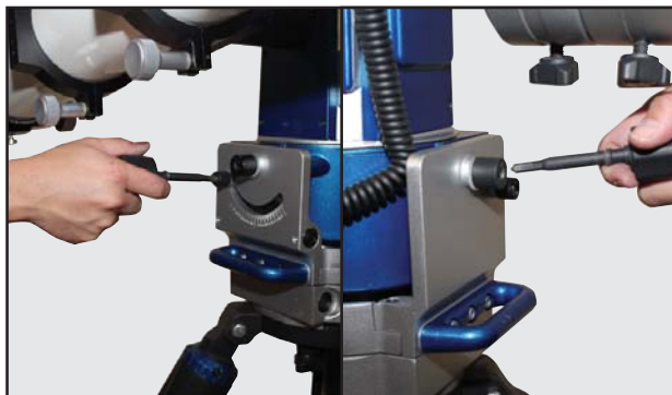
Fig 28: Loosen RA lock – right and left sides
