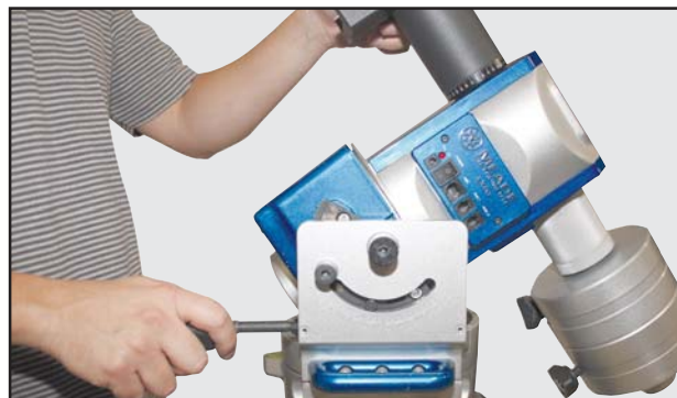
Fig 29: Tilting the mount head
