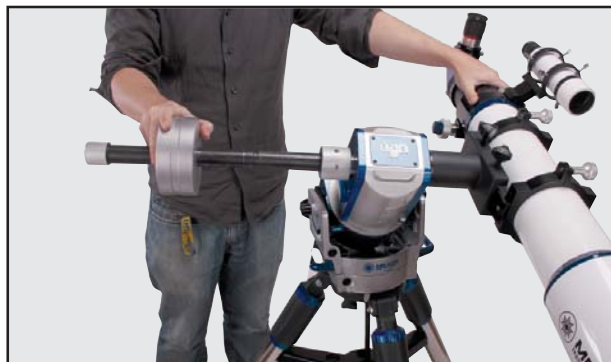
Fig 31: Adjust counterweight to achieve balance
