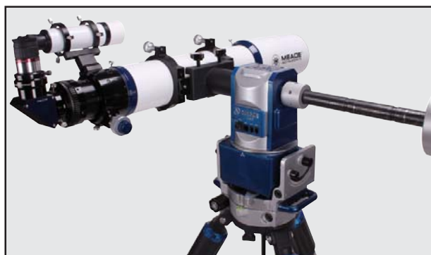
Fig 32: The Alt-Azimuth home position
