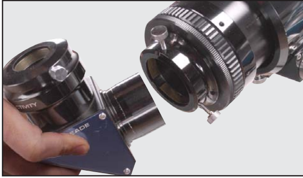
Fig 22: Secure diagonal into holder
