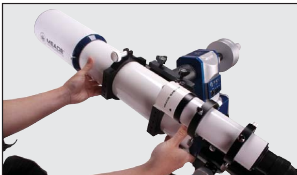
Fig 26: Balancing the OTA
