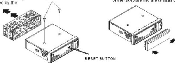
Push this reset button with a cuspidal object to renovate the distorted program once the program is distorted.
