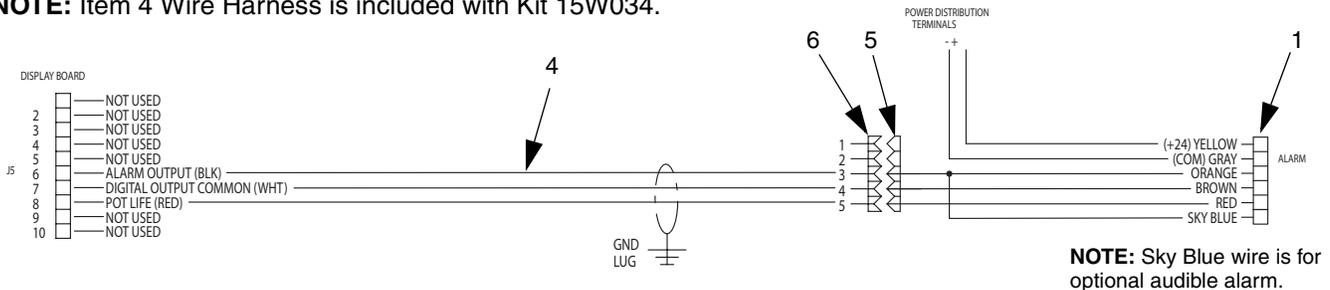
FIG. 6: 15W034 Beacon Tower Kit Wiring Diagram
