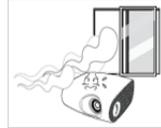
When a gas leak occurs, do not touch the product or the power plug and ventilate immediately.
