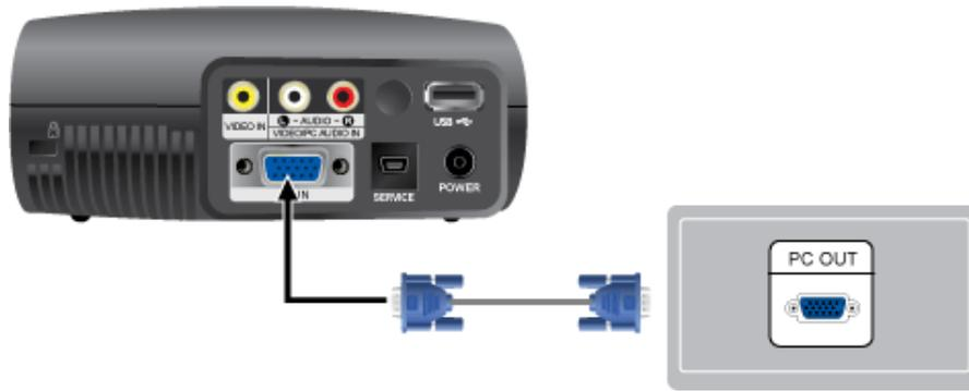
1. Connect [PC IN] port on the rear side of the projector to the monitor output port of the PC using a PC video cable.
