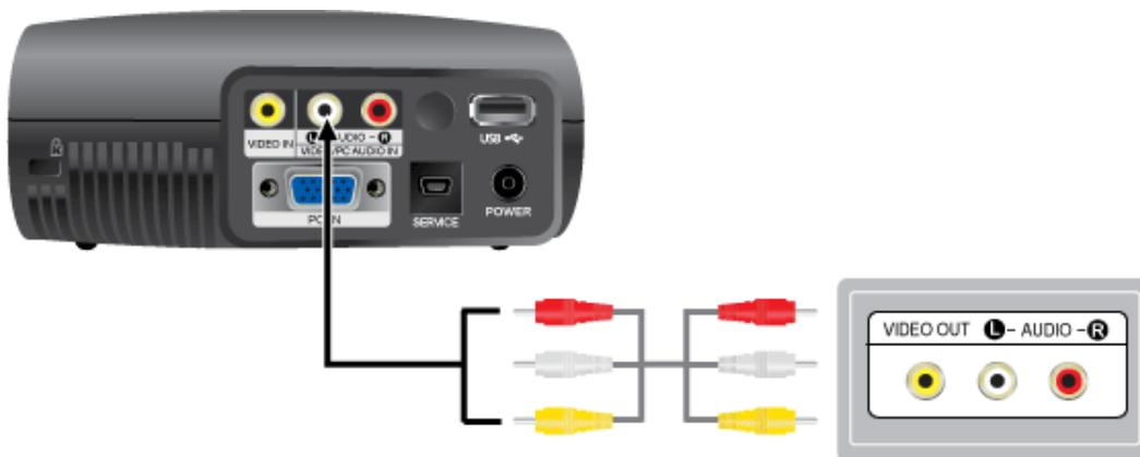
1. Connect [VIDEO IN(yellow)] input port of the projector to the VIDEO (yellow) OUT port of the video equipment using a video cable.
