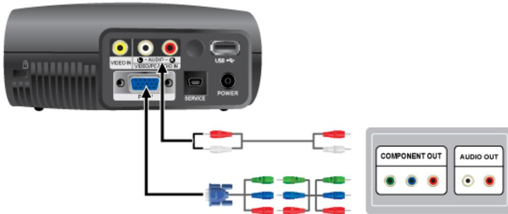
1. Connect [PC IN] input port on the rear of the projector to the COMPONENT port of AV equipment using a D-Sub/Component cable(Not supplied).
