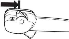
It is not allowed to set the stop switch in full throttle position.
