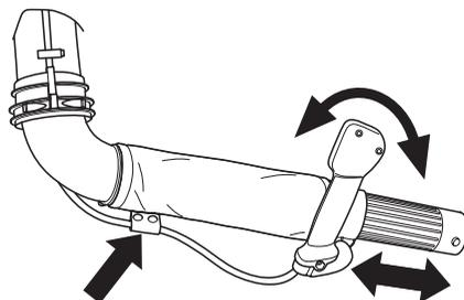
Connect the intermediate pipe and air nozzle. Push the pipes together and turn them so they lock in relation to one another.
