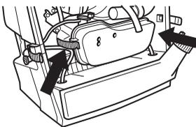
The air filter is fitted in the air filter cowling.
