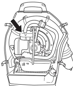
The muffler is equipped with a special spark arrestor mesh. The spark arrestor mesh should be cleaned once a month. This is best done with a wire brush.
