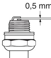
**CAUTION!** Always use the recommended spark plug type! Use of the wrong spark plug can damage the piston/cylinder.
