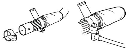
Assemble the intermediate pipe.
