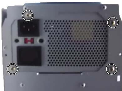
Fig. 23: Removing the power supply unit screws
