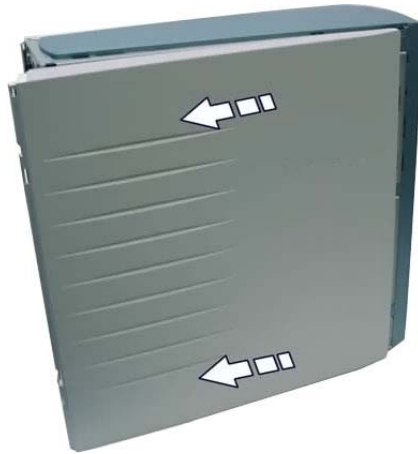
Fig. 3: Removing the left side cover
