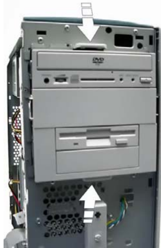
Fig. 7: Removing the drive bracket
