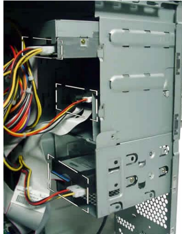
Fig. 5: Disconnecting power and data cables
