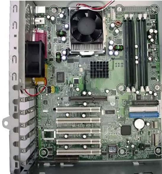
Fig. 22: Removing the screws of the motherboard
