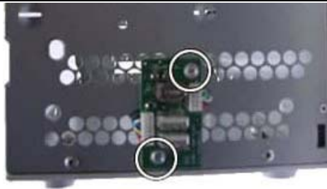
Fig. 14: Removing the front USB port screws
