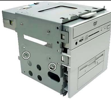
Fig. 9: Removing the floppy disk drive screws
