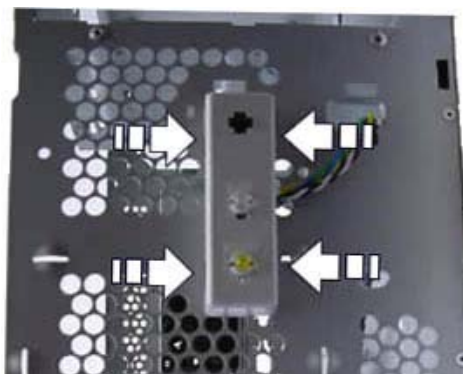
Fig. 15: Removing the switch/LED assembly
