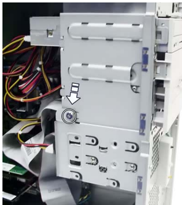
Fig. 6: Removing the drive bracket screw
