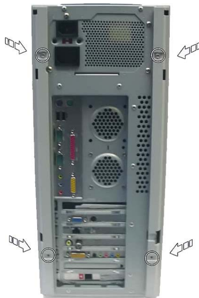
Fig. 2: Removing the left side cover screws
