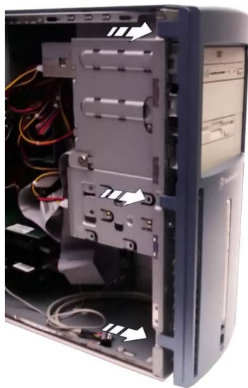
Fig. 4: Removing the front bezel
