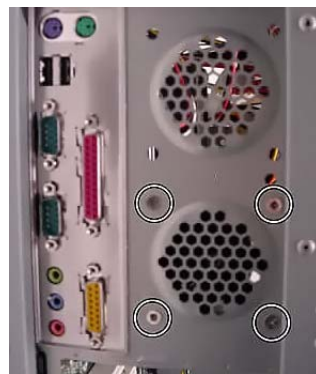
Fig. 20: Removing system fan screws
