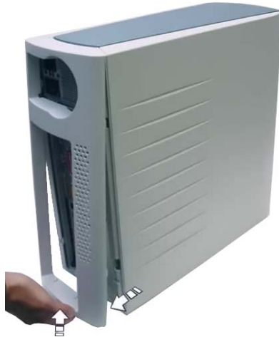
Fig. 1: Removing the rear bezel
