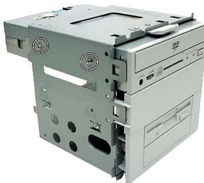
Fig. 8: Removing the DVD/CD-ROM drive screws
