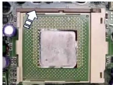
Fig. 17: Removing the CPU
