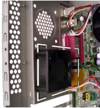
Fig. 19: Removing the system fan
