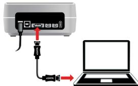
c) **eSATA:** Connect the eSATA cable to the eSATA port on the HD Dock Quattro (for data transfer with eSATA).
