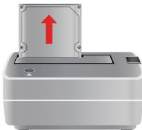
Gently remove the hard drive off in vertical direction.
