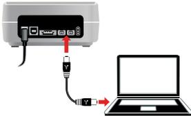
b) **Firewire 400/800:** Connect the Firewire cable to the Firewire port on the HD Dock Quattro (for data transfer with Firewire).
