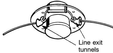
7. Correctly installed line will be the same length on both ends.
