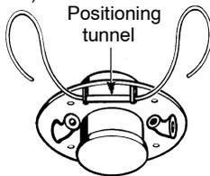
5. Insert ends of line one at a time through the line exit tunnels.
