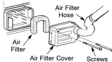
**NOTE:** Do not clean filter in gasoline or other flammable solvent to avoid creating a fire hazard or producing harmful evaporative emissions.
