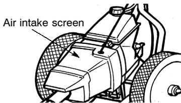
**WARNING:** Stop your unit before attempting to clean the intake screen. DO NOT USE GARDEN HOSE OR PRESSURE WASHER TO CLEAN THIS UNIT!
