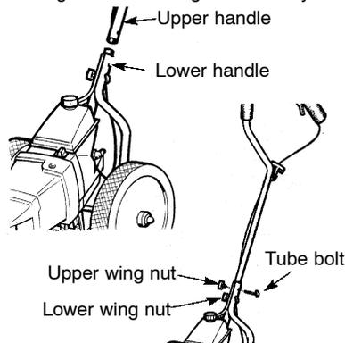
**NOTE:** When performing the following step, be sure the starter rope is not caught under the cable clamps. **The starter rope must hang freely to operate properly.**
