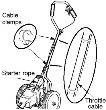
7. Align one cable clamp above the tube bolts and the other below the starter rope handle. Install the cable clamps one at a time around the tube and throttle cable.
