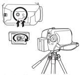
When the tripod is used, the card slot cover cannot be opened. Insert an SD card before attaching this unit to the tripod. (→ 22)
