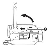
3 Insert/remove the SD card into/ from the card slot.
