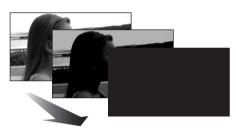
The image/audio gradually disappears. After the image/audio completely disappears, recording stops.
