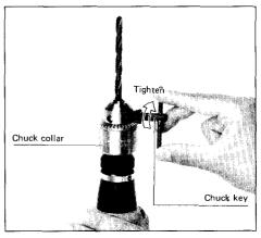
To remove the drill bit, place the chuck key into the chuck hole and turn counterclockwise.
