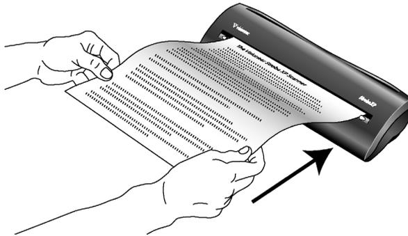
The scanner grabs the top edge of the paper and automatically begins to scan and feed the paper through the scanner.
