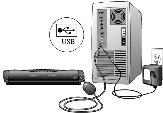
The USB symbol identifies the location of the USB port on your computer. If the plug does not attach easily, make sure that you are plugging it in correctly. Do not force the plug into the connection.
