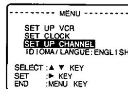
② ◀▶ Push ▲▼ to select "SET UP CHANNEL," and then push ▶ to display the "SET UP CHANNEL" screen.
