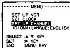
2 Push ▲▼ to select "SET UP CHANNEL," and then push ► to display the "SET UP CHANNEL" screen.
