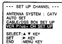
③ ◀▶ Push ▲▼ to select "VCR Plus+ CH SET UP," and then push ▶ to display the "VCR Plus+ CH SET UP" screen.
