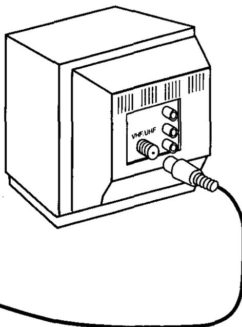
RF Coaxial Cable (VCR-TV Connection Cable) (supplied)
