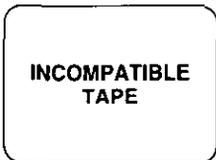
When an incompatible tape is detected, "INCOMPATIBLE TAPE" will appear for 5 seconds.
