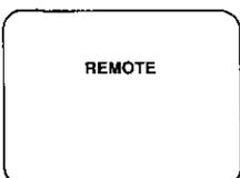
When the Palmcorder and remote are not set to the same mode (VCR1 or VCR2), "CHECK REMOTE MODE" will also appear for 5 seconds when the Palmcorder is first turned on.
