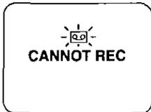
When Audio dub is performed and the sliding record tab is open, or a blank portion of tape is detected, "⏏" will flash and "CANNOT REC" will appear for 5 seconds.
