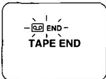
When the tape is about to end in REC mode, "⏏END" will flash and "TAPE END" will appear for 5 seconds.
