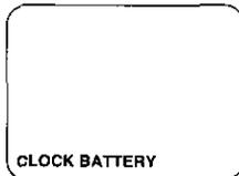
— When the built-in lithium clock battery is discharged, "CLOCK BATTERY" will appear. To re-charge the lithium clock battery, connect the AC Adaptor to the Palmcorder. Recharging takes approx. 4 hours. Reset the clock after charging.
