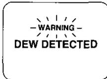
— If excessive moisture condenses in the unit, "WARNING" will flash, "DEW DETECTED" will appear, and the Palmcorder will automatically turn OFF in 15 seconds. In this case, wait until the indicator no longer flashes when your Palmcorder is turned on again.
