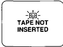
If the Palmcorder is in CAMERA mode without a cassette inserted, "⏏" will flash and "TAPE NOT INSERTED" will appear for 5 seconds. Recording will not start.
