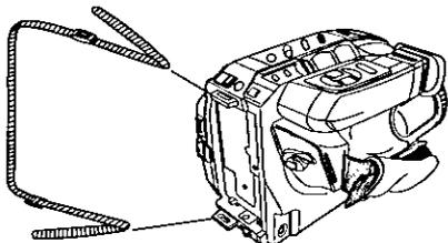
**2** Thread strap ends through Strap Rings on Camcorder.
