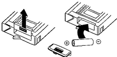
Remove Battery lid and insert AA battery.
