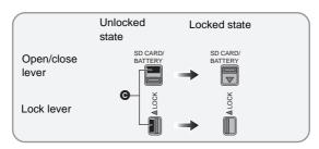
Lock securely to the points where the red portion of the open/close lever and LOCK lever are no longer visible.
