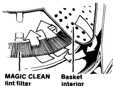
The lint filter at the bottom of the washer basket cleans itself. During agitation, wash and rinse water pass over the filter, separating lint from water. The collected particles of lint are then continuously spun away from the filter and washed out of the system at the end of the wash cycle.
