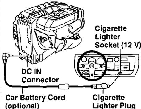
**1** Connect **PV-C16 Car Battery Cord (optional)** to **Camcorder DC IN**.
