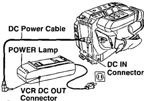
**1** Connect **AC Adaptor VCR DC OUT** to **Camcorder DC IN** with supplied **DC Power Cable**.
