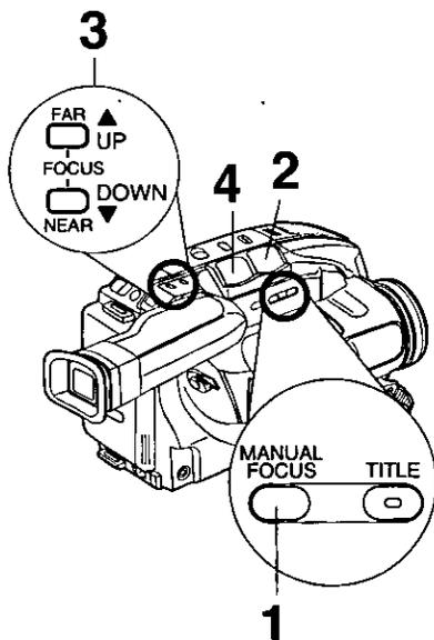
**1** Press **MANUAL FOCUS** so "MF" (Manual Focus) appears in EVF or LCD monitor.
