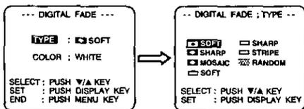
**4** Press **DISPLAY** for DIGITAL FADE menu. Press **DOWN ▼** to select **COLOR**. Press **DISPLAY** for COLOR menu. Press **UP ▲** or **DOWN ▼** to select from 8 colors.
