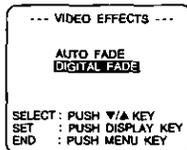
**3** Press **DISPLAY** for DIGITAL FADE menu. Press **UP ▲** or **DOWN ▼** to select **TYPE**. Press **DISPLAY** for TYPE menu. Press **UP ▲** or **DOWN ▼** to select from 7 different types of fades.
