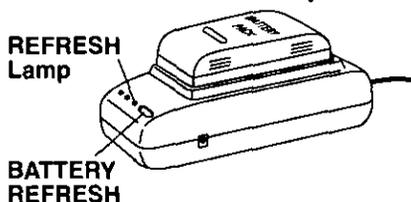
To use battery refresh, insert Battery on AC Adaptor (see steps 1-2 above), then press **BATTERY REFRESH**.
