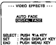
**3** Press **DISPLAY** for DIGITAL FADE menu. Press **UP ▲** or **DOWN ▼** to select **TYPE**. Press **DISPLAY** for TYPE menu. Press **UP ▲** or **DOWN ▼** to select from 7 types.
