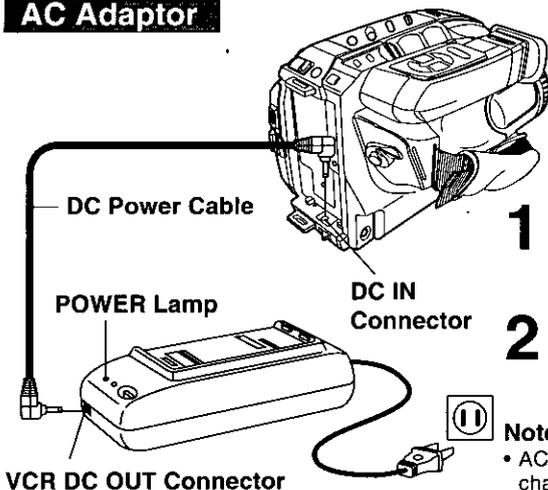
**1** Connect **AC Adaptor VCR DC OUT** to **Camcorder DC IN** with supplied DC Power Cable.
