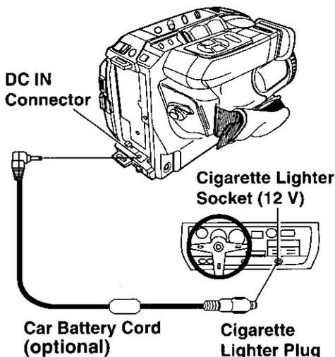
**1** Connect **PV-C16 Car Battery Cord (optional)** to **Camcorder DC IN**.
