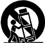
Use only with a cart, stand, tripod, bracket, or table recommended by the manufacturer, or sold with the video unit. Any mounting of the unit should follow the manufacturer's instructions and should use a mounting accessory recommended by the manufacturer. An appliance and cart combination should be moved with care. Quick stops, excessive force, and uneven surfaces may cause the appliance and cart combination to overturn.
