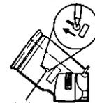
**2** Press (A) with a sharp end tip like a ball point pen or mechanical pencil and slide in direction of arrow
