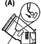
**3** Remove any lint or dust from the access hole with canned air or other air blower
