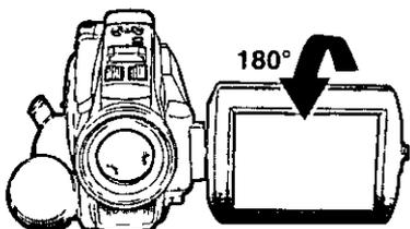
Rotate the LCD monitor 180 degrees so it faces the same direction as the lens to record yourself (CAMERA mode)
