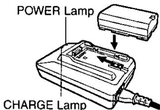
**1** Connect and plug in the Power Cord as shown
