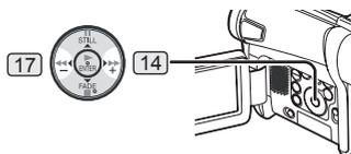
If the [▶▶] Button **14** or [◀◀] Button **17** is pressed during Playback, it turns to Cue Playback **A** or Review Playback **B**.
