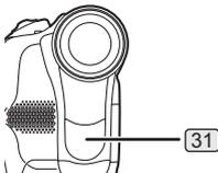
• Do not cover the White Balance Sensor with your hand during recording because White Balance will not function normally.
