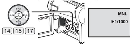
**3 Press the [▶▶] Button (14) or [◀◀] Button (17) to adjust the shutter speed.**
