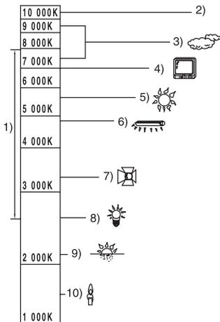
Outside of the effective range of Automatic White Balance Adjustment, the image will become reddish or bluish. Even within the effective range of Automatic White Balance Adjustment, the Automatic White Balance Adjustment may not function properly if there is more than one light source. In this case, adjust the White Balance.
