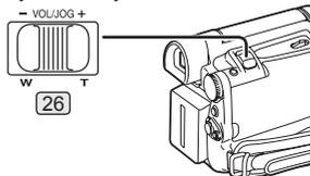
To adjust the volume with the Remote Control, press the [T] or [W] Button to display the [VOLUME] Indication. Press the [T] Button to increase the volume or press the [W] Button to decrease the volume. The [VOLUME] indication disappears immediately after adjustment is made.
