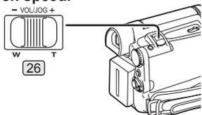
The following 6 playback speeds are available for the Variable Speed Search Function in both the fast-forwarding and rewinding directions: 1/5x (slow playback in SP Mode only), 1/3x (slow playback in LP Mode only), 1x, 2x, 5x, 10x and 20x.
