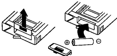
Remove the Battery Compartment lid and insert the AA size battery.
