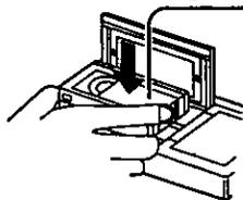
**3** Insert the **VHS** cassette with the window facing up and to the left. Then, snap the lid shut.
