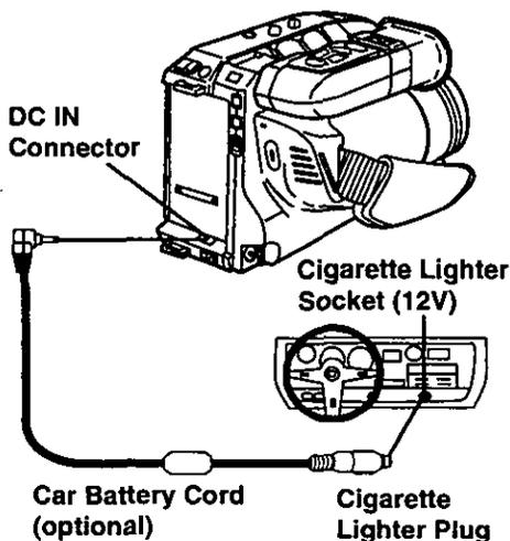
**1** Connect a PV-C16 Car Battery Cord (optional) to the DC IN of the Palmcorder.
