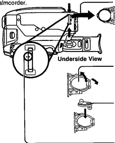
**1** While pinching the stopper tabs, pull the tray out of the Battery Compartment.
