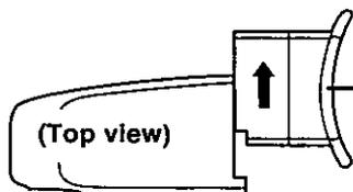
**2** Remove the eyepiece. (Do not twist.)
