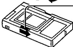
**2** Slide the **RELEASE** button in the direction of the arrow to open the PlayPak door.
