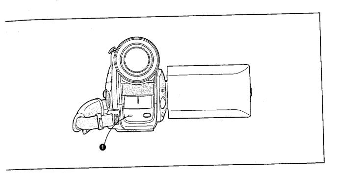
Tally Lamp 1 If you don't want the Tally Lamp to light during recording, set [TALLY LAMP] on the [CAMERA SETUP] Sub-Menu to [OFF].
