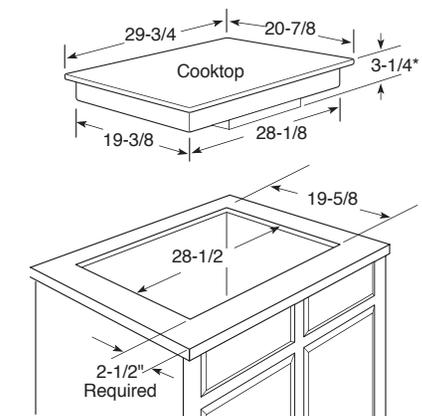
\*Depth of unit at conduit location (right rear) is 4-5/8"
