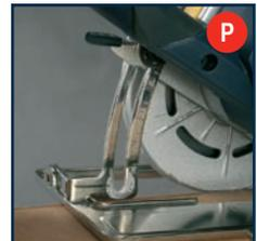
4. Tighten the depth locking lever (13) by pushing the lever upwards (Fig. N).
