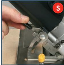
4. Tighten the bevel adjustment lever (8) to secure the base plate.
