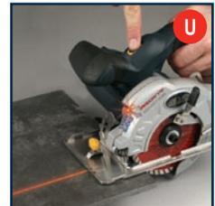
4. Switch on the laser beam using the laser light on/off button (4) (Fig. U).
