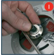
**IMPORTANT.** After replacing the saw blade, make sure that the saw blade runs freely by turning the blade by hand. Check that the directional arrow on the saw blade points clockwise when viewed from the mounting side.
