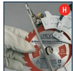
8. Mount the new saw blade onto the spindle and against the inner flange (Fig. H).
