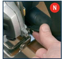
3. Hold the base plate flat against the edge of the work piece and lift the body of the saw until the blade is at the right depth (Fig. O & P). Use the depth of cut indicator (14) to determine the cutting depth.
