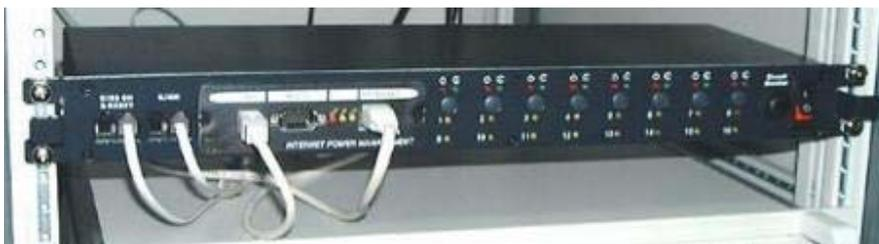
The Remote Power Manager (iSwitch) is a network-manageable, intelligent power control unit designed to provide control of power for up to eight electrical devices.
