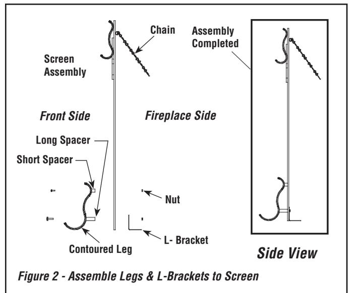
Figure 2 - Assemble Legs & L-Brackets to Screen
