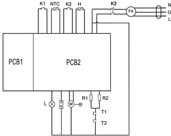
FA-Electromagnetic interference inhibitor
