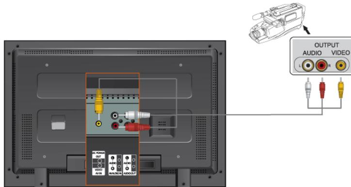
1. Locate the AV output jacks on the camcorder. They are usually found on the side or back of the camcorder. Connect a set of audio cables between the AUDIO OUTPUT jacks on the camcorder and the AV AUDIO IN [L-AUDIO-R] on the LCD Display .
