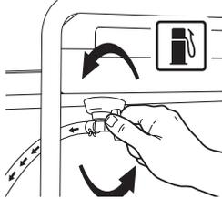
2. Move the choke control located on the engine to the "Choke" position.
