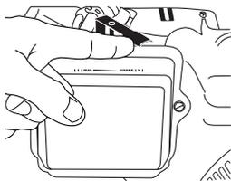
**NOTE:** No choke is required on warm engines. make sure choke is in the "RUN" position on warm engine starts.
