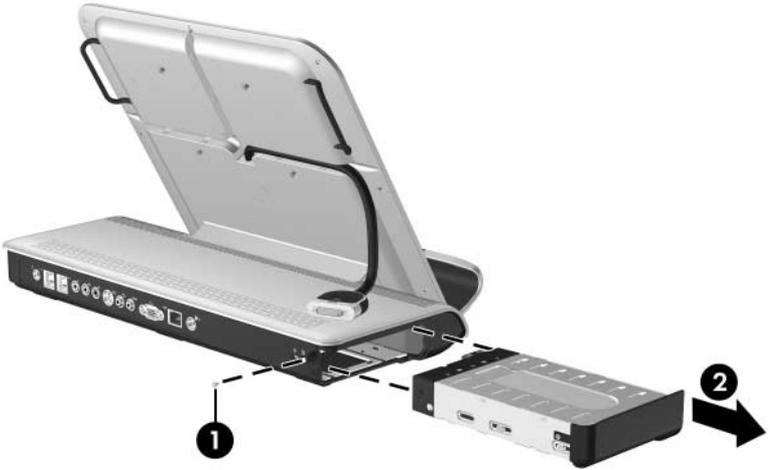
*Removing the Hard Drive Carrier*
