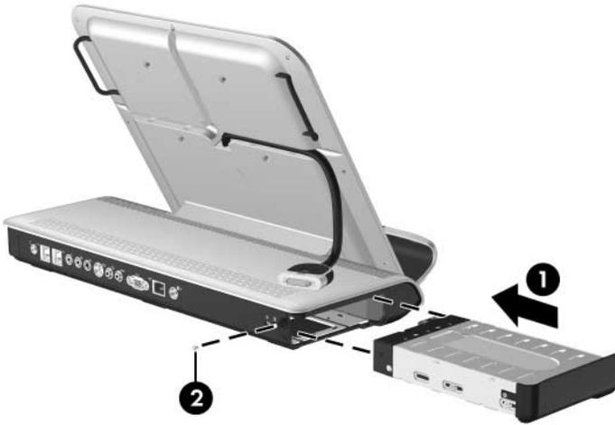
*Installing the Hard Drive Carrier*
