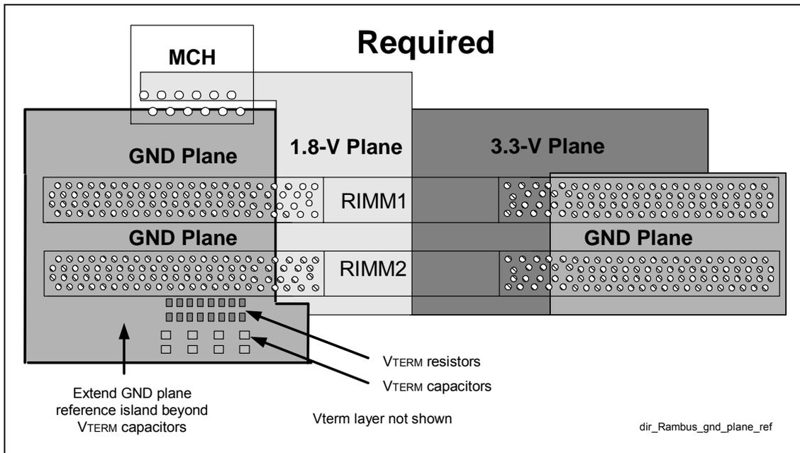
The ground reference island under the RSL signals **MUST** be connected to the ground pins on the RIMM connector and the ground vias used to connect the ground isolation on the first and fourth layers.
