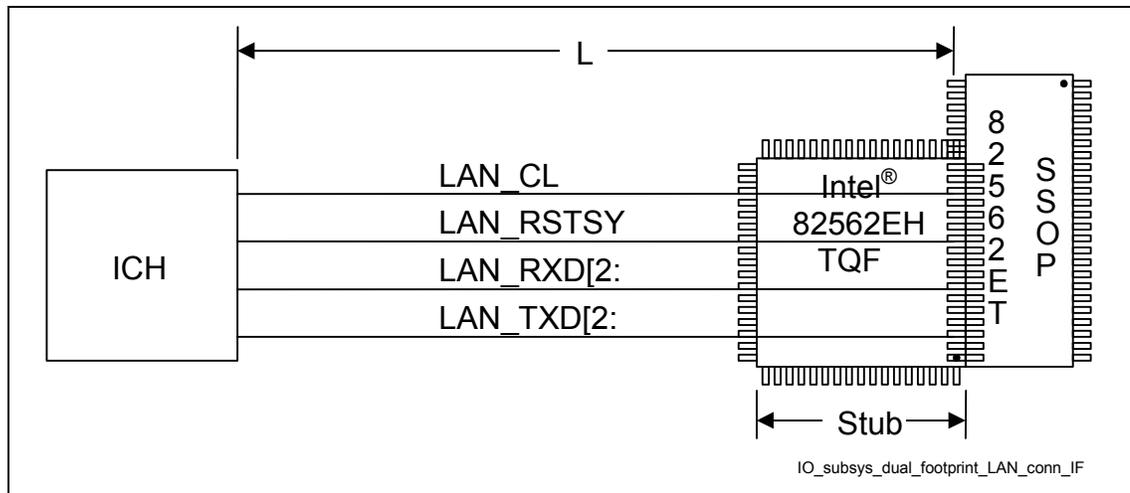
**Figure 77. Dual-Footprint Analog Interface**
