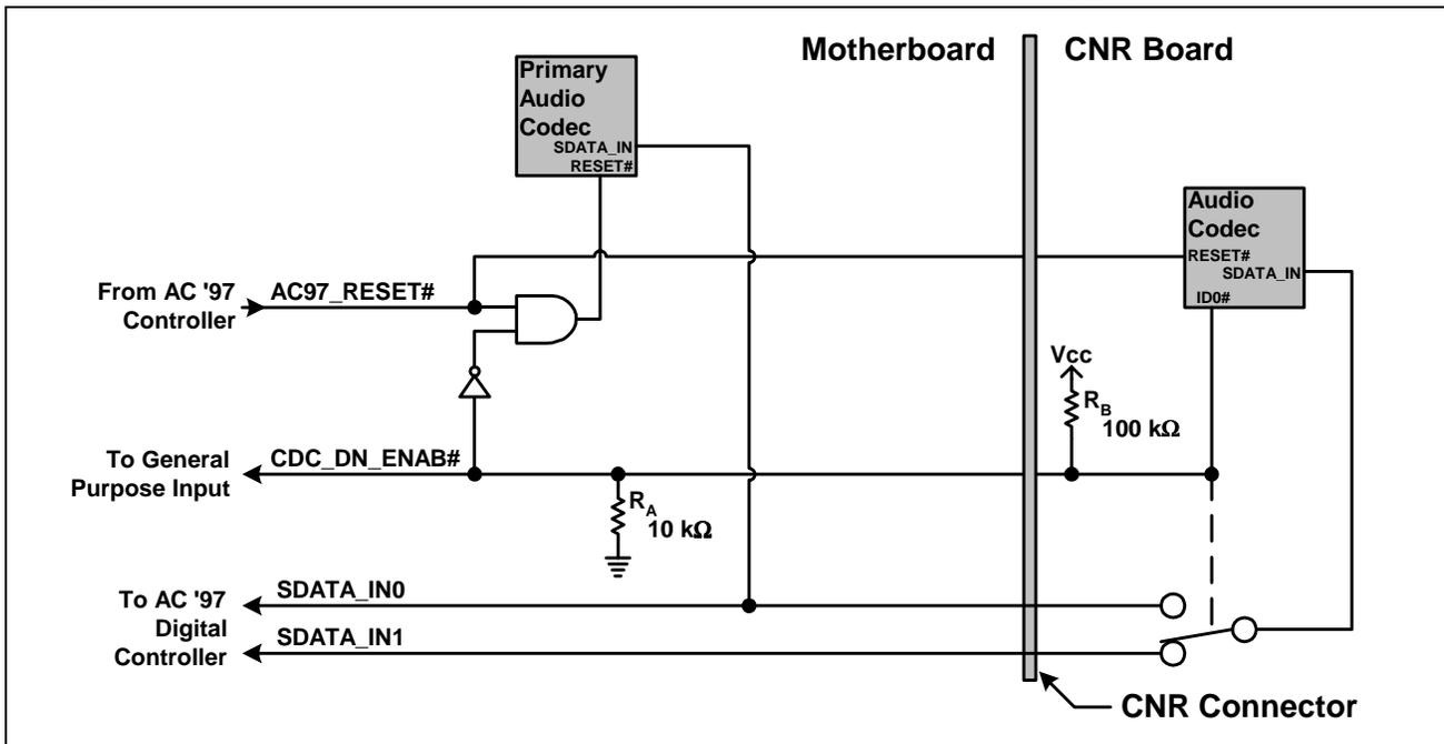
Figure 52 shows the circuitry required on the motherboard to support a two-codec down configuration. This circuitry disables the codec on a single codec CNR. Notice that in this configuration the resistor,  $R_B$ , has been changed to 100 k $\Omega$ .
