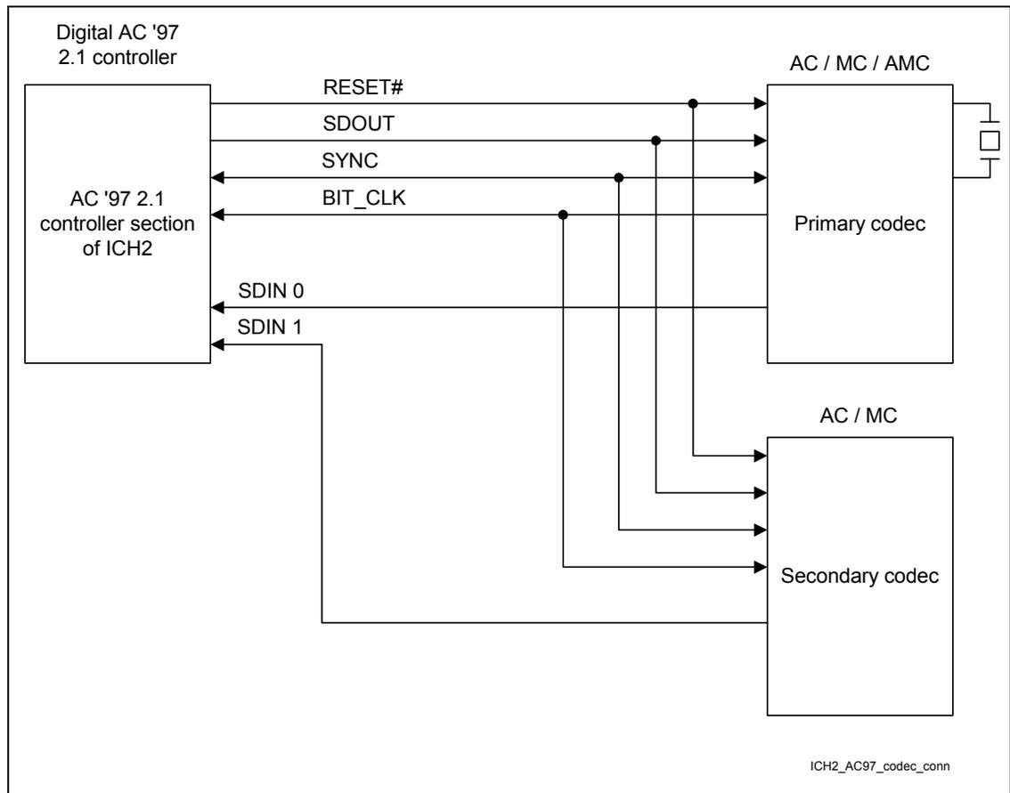
The AC'97 interface can be routed using 5 mil traces, with 5 mil space between traces. The maximum length from ICH2 to CODEC/CNR is 14 inches, in a tee topology. This assumes that a CNR riser card implements its audio solution with a maximum trace length of 4 inches for the AC-link. The trace impedance should be as follows:  $Z_0 = 60 \Omega \pm 15\%$ .
