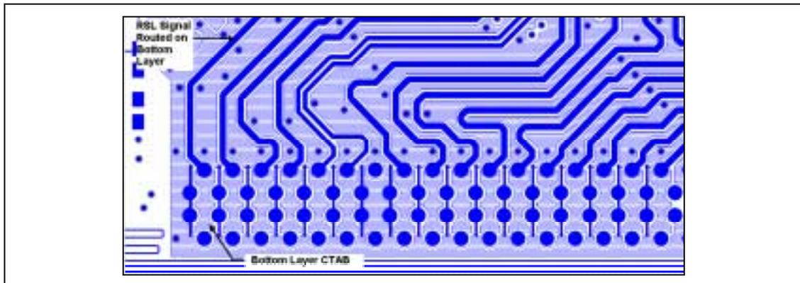
The CTAB can be implemented on the multiple layers to minimize routing and space constraints. Figure 28 shows the use of CTABs on the top and bottom layer for bottom-layer RSL and clocking signals routed between RIMMs.
