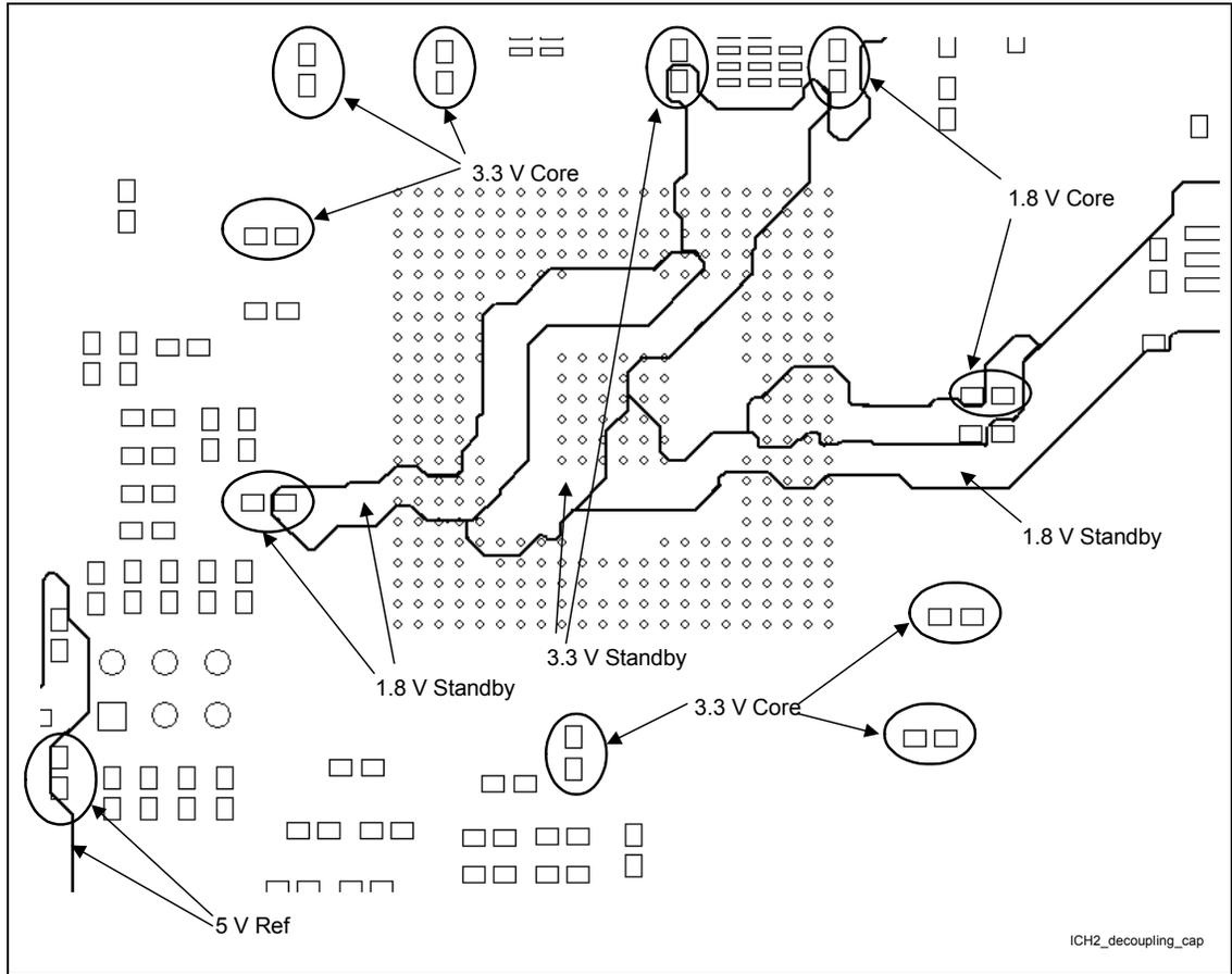
The previous figure shows the layout of the ICH2 decoupling capacitors for various power planes around the ICH2. The decoupling caps are circled, with an arrow pointing to the power plane/trace to which they are connected.
