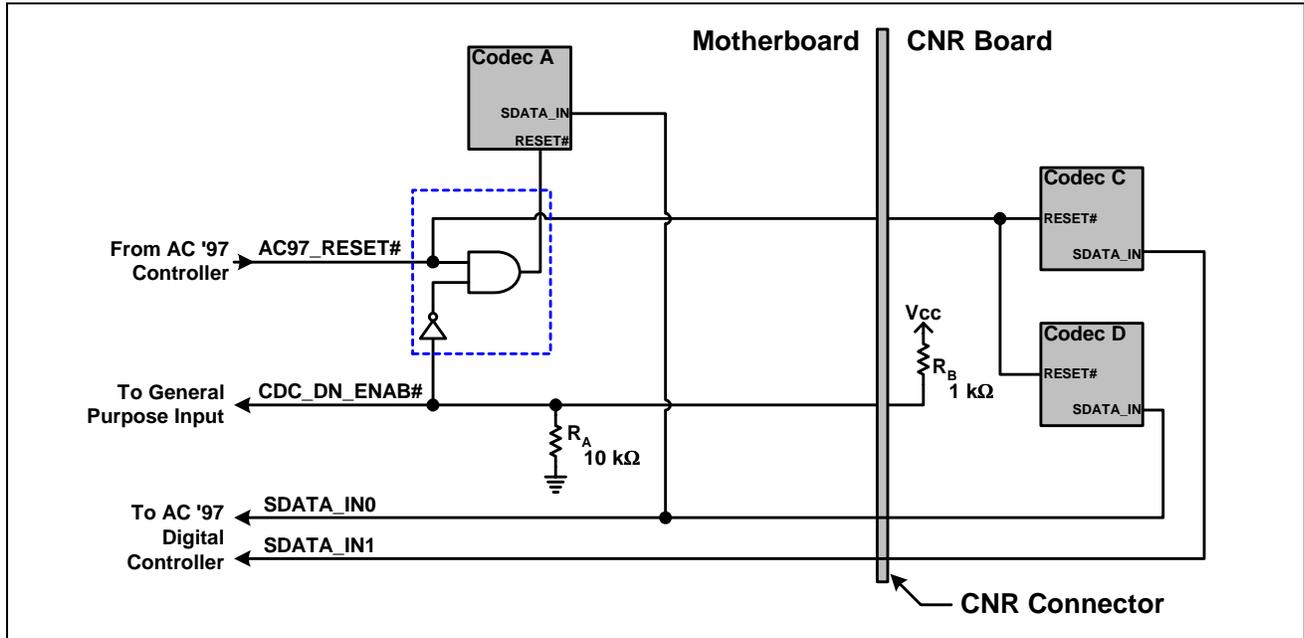
As shown in Figure 51, when a single codec is located on the motherboard, the resistor  $R_A$  and the circuitry (AND and NOT gates) shown inside the dashed box must be implemented, on the motherboard. This circuitry is required in order to disable the motherboard codec when a CNR is installed which contains two AC '97 codecs (or a single AC '97 codec which must be the primary codec on the AC-Link).
