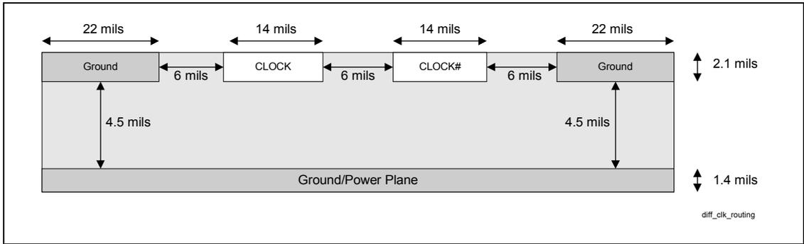
**Figure 92. Non-Differential Clock Routing Diagram (Section B)**
