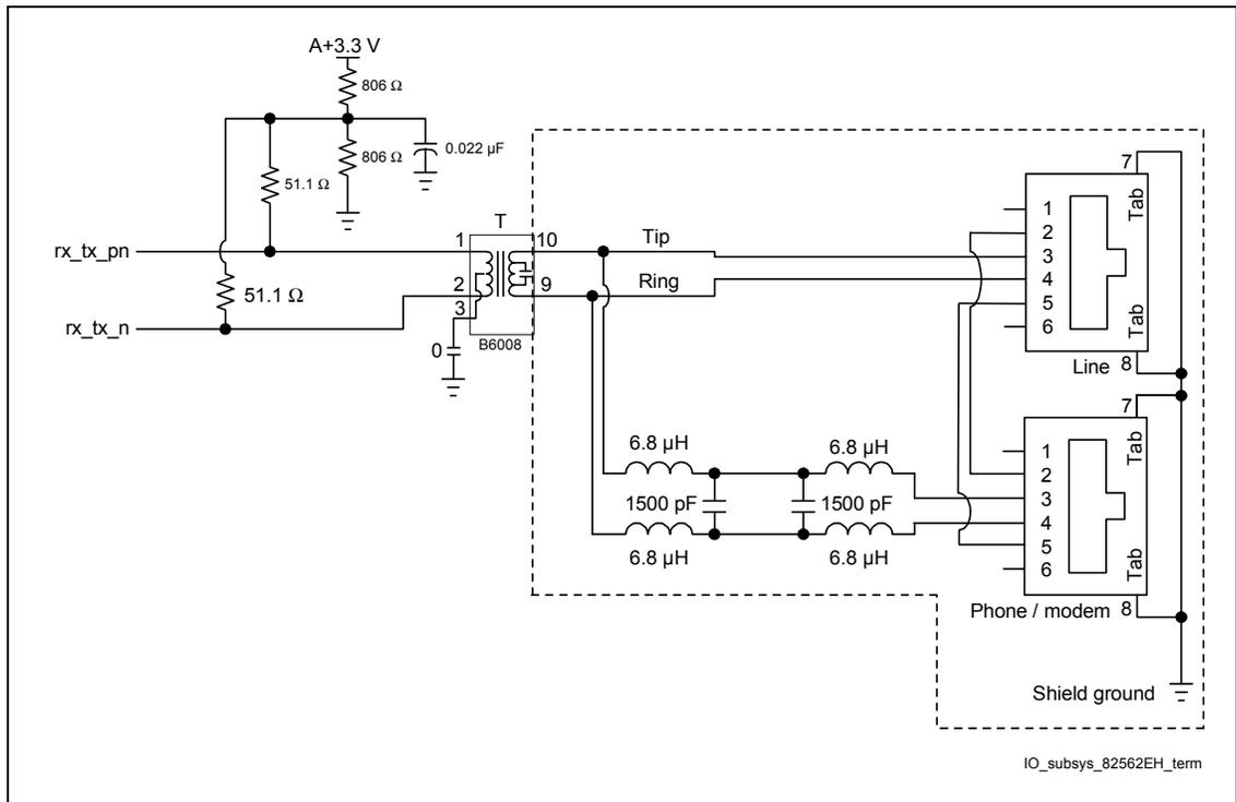
The filter and magnetics component T integrates the required filter network, high-voltage impulse protection, and transformer to support the HomePNA LAN interface.
