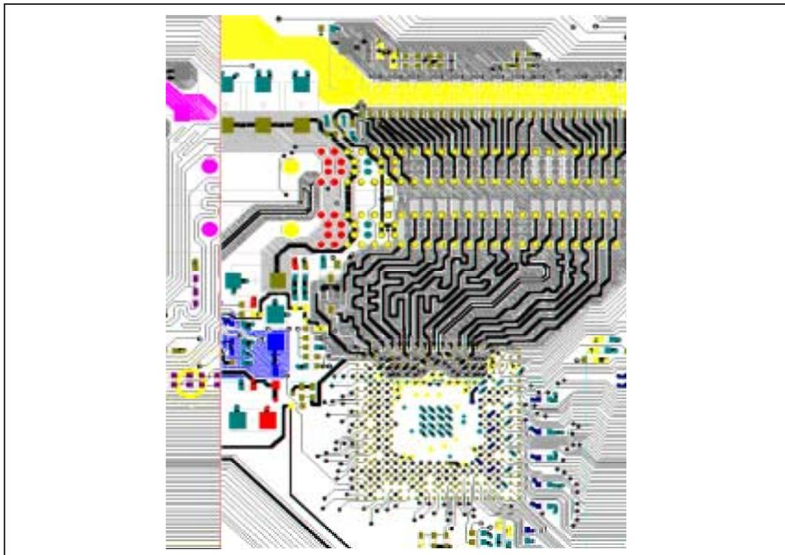
Figure 16. Secondary-Side RSL Breakout Example
