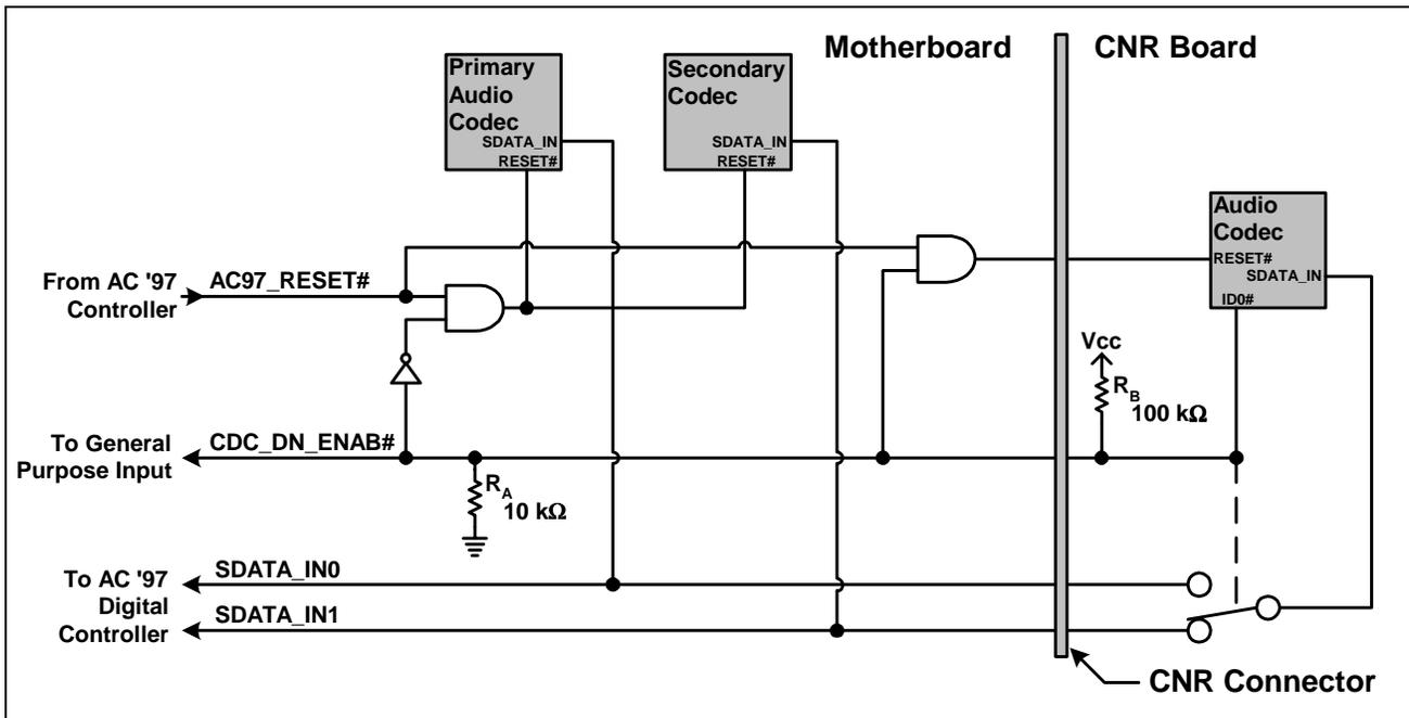
Figure 53 shows the case of two-codex down and a dual-codec CNR. In this case, both codex on the motherboard are disabled (while both on CNR are active) by  $R_A$  being 10 k $\Omega$  and  $R_B$  being 1 k $\Omega$ .
