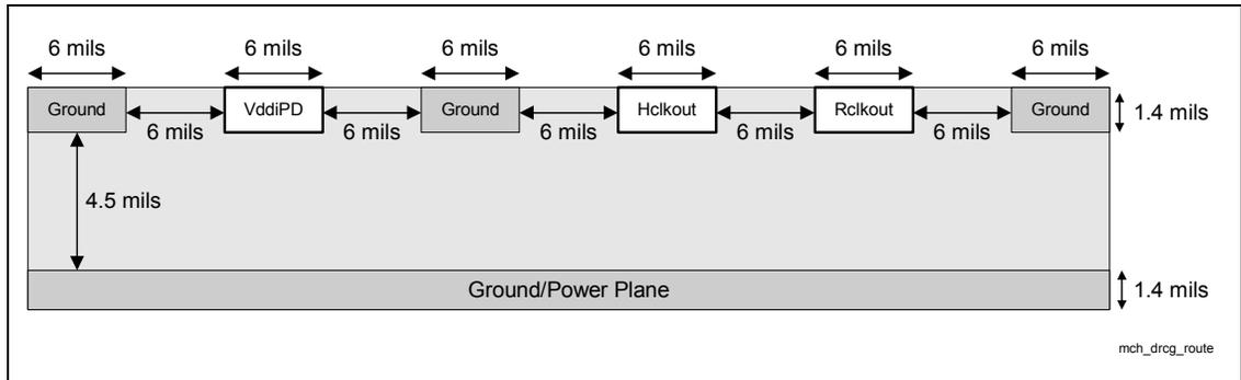
Hclkout, Rclkout, and VddIPD should be routed as shown in Figure 89. Note that the VddIPD pin can be connected directly to 1.8 V near the DRCG, if the 1.8 V plane extends near the DRCG. However, if a 1.8 V trace must be run, it should originate at the MCH and be routed as shown.
