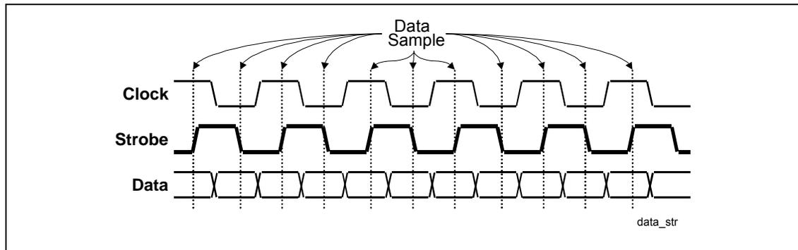
For a source-synchronous-strobed interface, it is **very important** that the strobe signals be routed carefully. These signals must be very clean (i.e., free of noise). Data signals typically are latched on the rising or falling edge of the strobe signal (or both). If there is noise on these signals, it could cause an extra “edge” to be detected, thus latching incorrect data. Refer to the following example figures.
