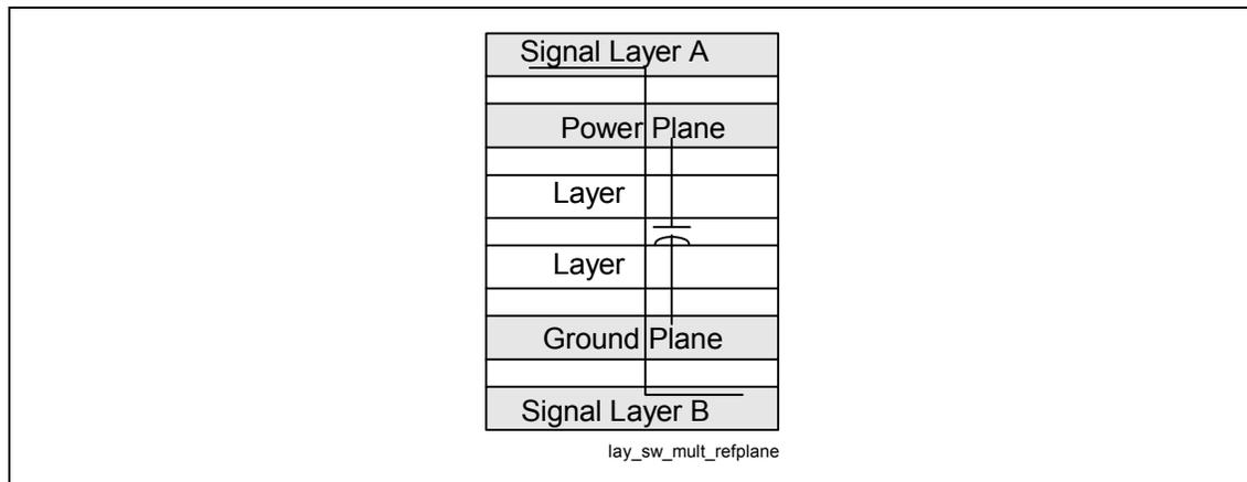
Figure 83. One Layer with Multiple Reference Planes
