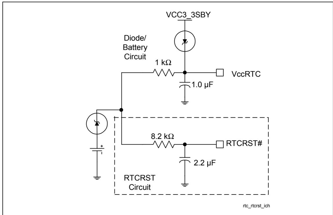
This RTCRST# circuit is combined with the diode circuit (Figure 60. Diode Circuit Connecting RTC External Battery), which allows the RTC well to be powered by the battery when system power is unavailable. Figure 59 is an example of the circuit used in conjunction with the external diode circuit.
