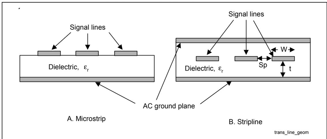
Additional aggressors are possible in the z-direction, if adjacent signal layers are not routed in mutually perpendicular directions. Because crosstalk coupling coefficients decrease rapidly with increasing separation, it is rarely necessary to consider aggressors at least five line widths away from the victim. The maximum crosstalk occurs when all aggressors are switching in the same direction at the same time.
