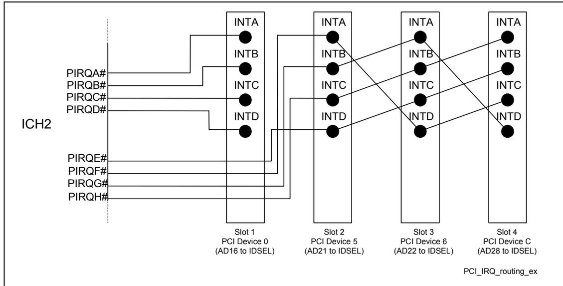
The PCI IRQ routing in the previous figure allows the ICH2’s internal functions to have a dedicated IRQ, assuming add-in cards are single-function devices and use INTA. If a P2P bridge card or a multifunction device uses more than one INTn# pin on the ICH2 PCI bus, the ICH2’s internal functions will start sharing IRQs.
