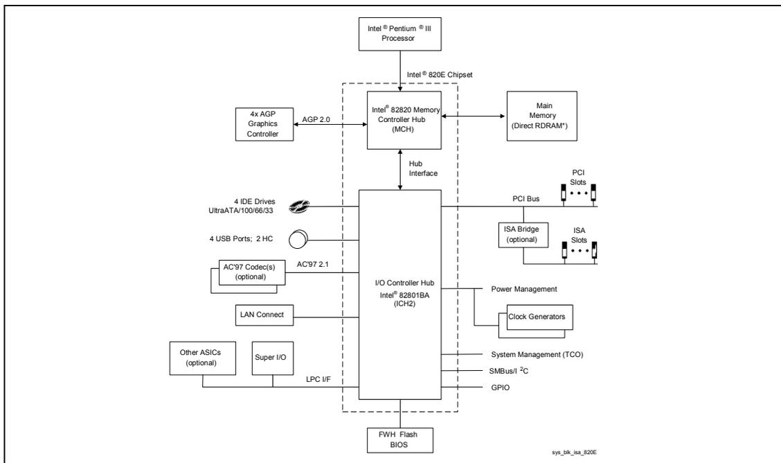
Figure 3. Intel® 820E Chipset Platform Dual-Processor Performance Desktop Block Diagram
