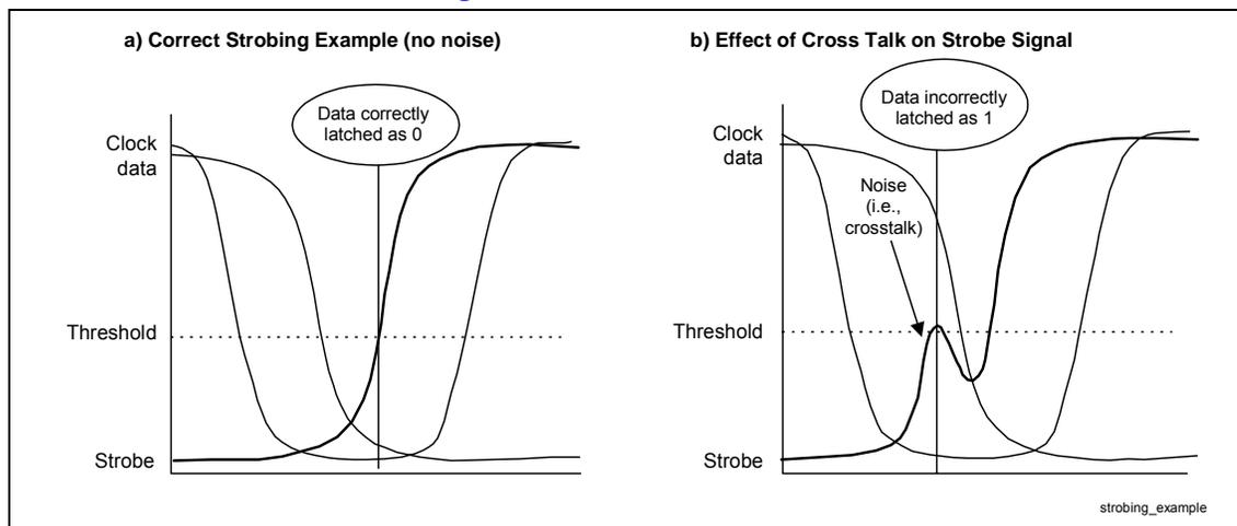
Some buses have more than one strobe (i.e., AGP). The AGP 1.0 specification (1× and 2× modes) employs three strobe signals, each of which is used to strobe different data signals (i.e., each strobe has an associated set of data signals). The associations for AGP 1.0 (AGP 2×) are listed in the following table. Refer to Section 2.8 for more information on AGP 2.0 (AGP 4×, 1.5 V).
