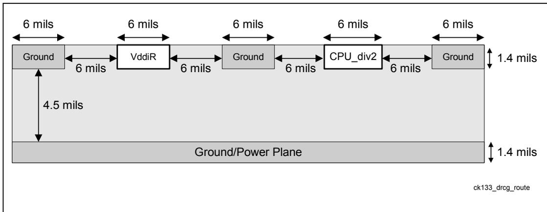
VddIR and CPU\_div2 must be routed as shown in Figure 88. Note that the VddIR pin can be connected directly to 2.5 V near the DRCG if the 2.5 V plane extends near the DRCG. However, if a 2.5 V trace must be used, it should originate at the CK133 and be routed as shown.
