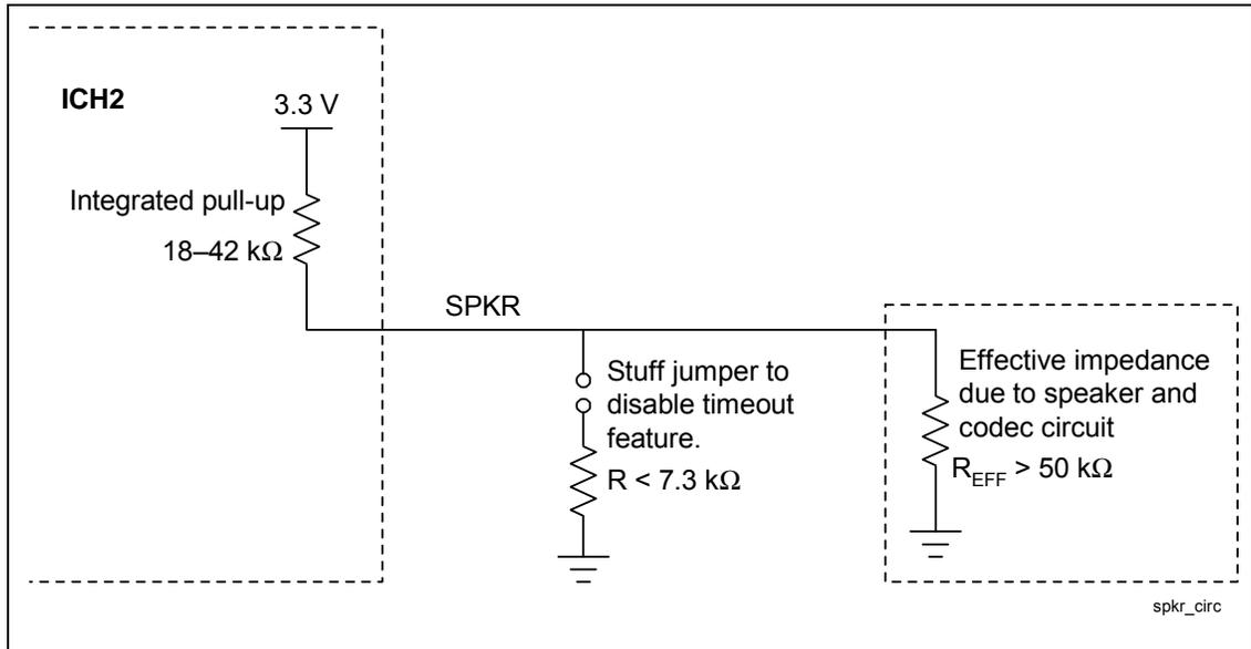
It should be noted that this is not the only solution to this problem. Board designers can also isolate the load from the SPKR pin until POWEROK is in a stable high state. This would allow a weak effective load to be implemented.
