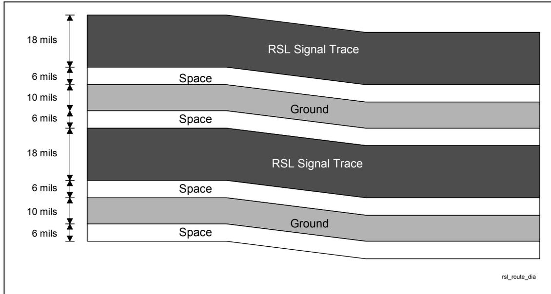
The following two figures show the top view of an example RSL breakout and route.
