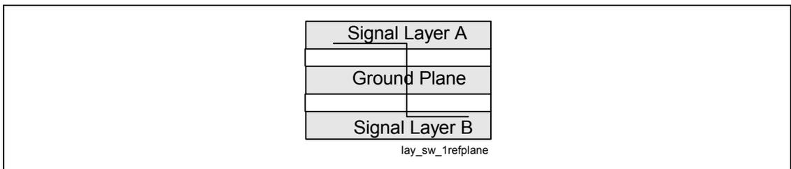
**Figure 81. Layer Switch with Multiple Reference Planes (Same Type)**
