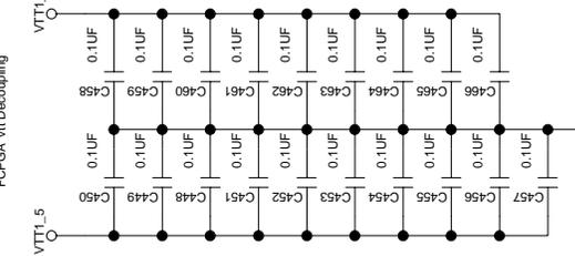
For chisel decoupling, use 0.1uF and 0.01uF decoupling capacitor at each corner of the device. If there is room, also add 0.01uF capacitor in the middle of each quad. Place additional caps if routable.
