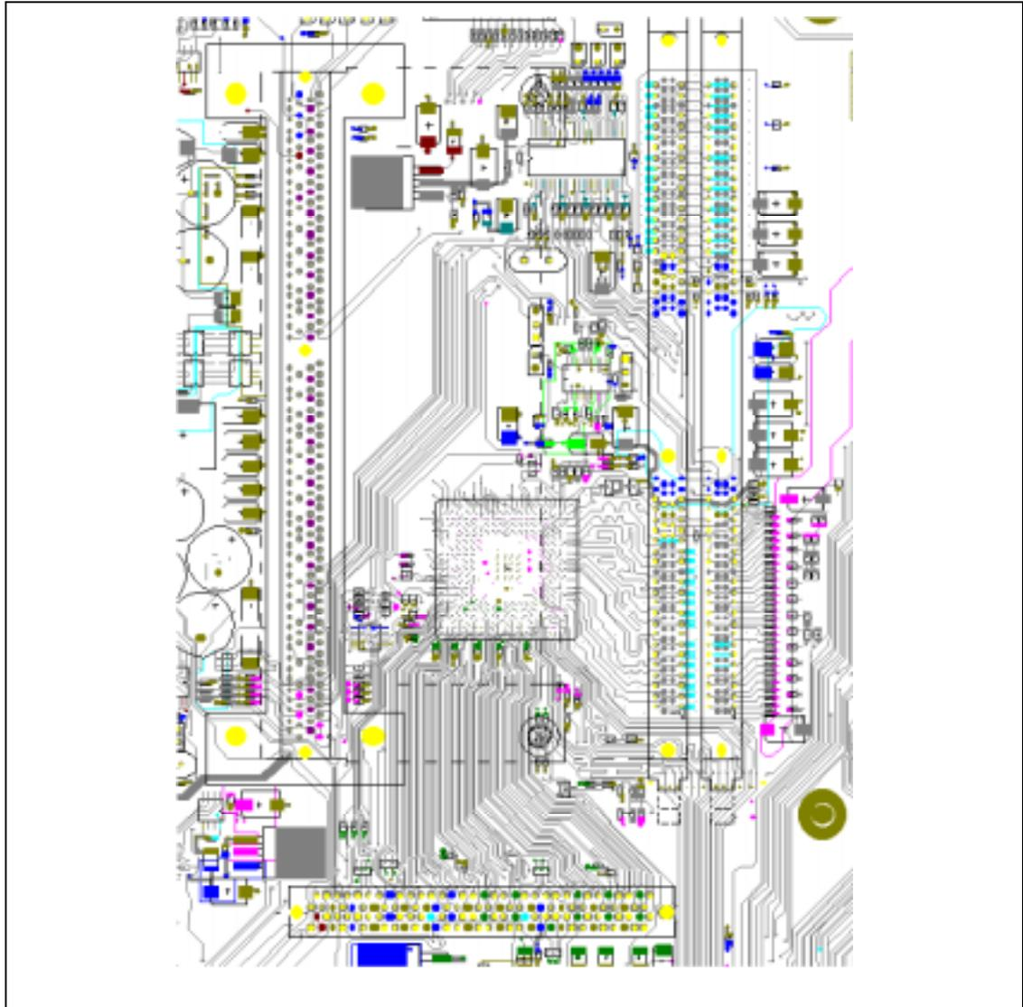
Figure 9. Secondary-Side MCH Core Routing Example (ATX)
