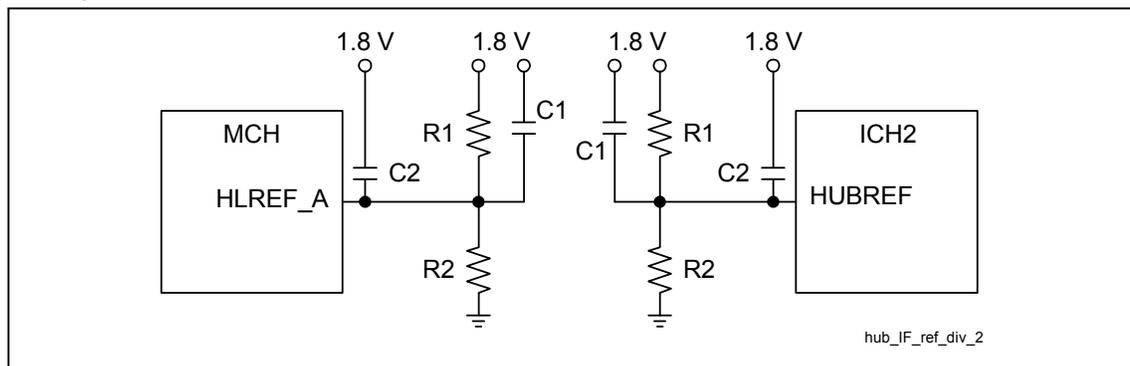
The resistor values, R1 and R2, must be rated at 1% tolerance. The selected resistor values ensure that the reference voltage tolerance is maintained over the input leakage specification. A 0.1  $\mu$ F capacitor (C1 in the previous circuits) should be placed close to R1 and R2. Also, a 0.01  $\mu$ F bypass capacitor (C2 in the previous circuits) should be placed within 0.25 inch of each HUBREF pin. The trace length from the divider circuit to the HLREF pin must be no longer than 3.5 inches.
