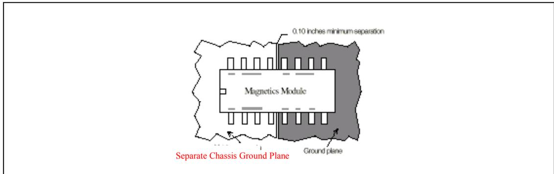
Good grounding requires the minimization of inductance levels in the interconnections. EMI radiation can be reduced significantly by keeping ground returns short, signal loop areas small, and power inputs bypassed to signal return.
