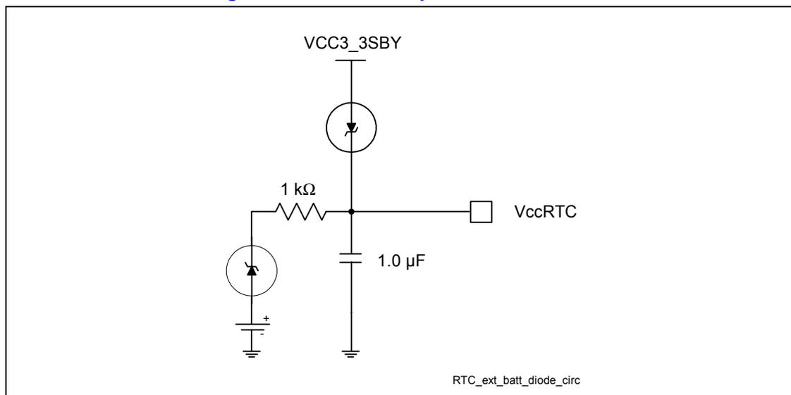
A standby power supply should be used in a desktop system to provide continuous power to the RTC when available, which will significantly increase the RTC battery life and thereby increase the RTC accuracy.
