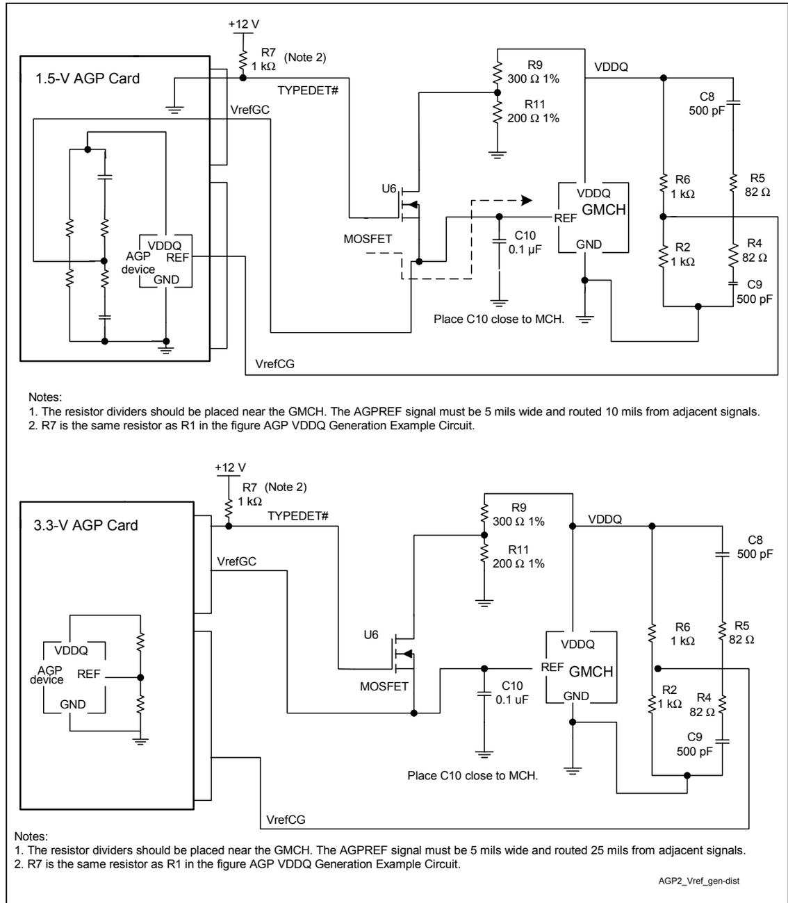
The flexible  $V_{REF}$  divider shown in the preceding figure uses an FET switch to switch between the locally generated  $V_{REF}$  (for 3.3 V add-in cards) and the source-generated  $V_{REF}$  (for 1.5 V add-in cards).
