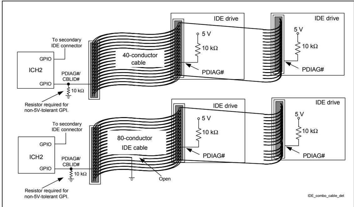
After diagnostics, this mechanism allows the BIOS to sample PDIAG#/CBLID#. If the signal is high, there is a 40-conductor cable in the system and ATA modes 3, 4 and 5 must not be enabled.
