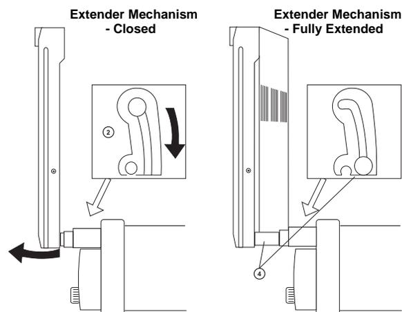
2. Locate the extender mechanism behind the screen.
