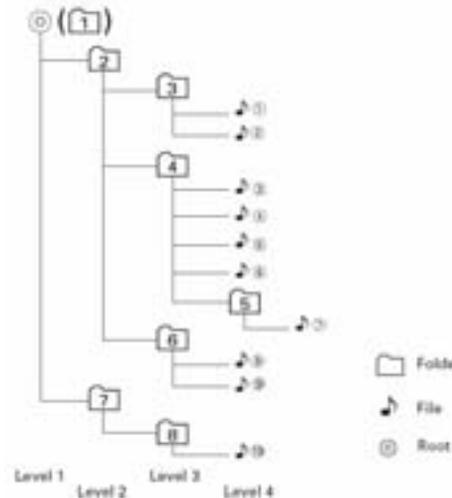
The VM9512 player will only recognize three folder levels and does not display folders containing only other folders. In the example above, the unit will display folders 3, 4, 6, and 8, but not 2 and 7 since they do not contain any tracks directly. Folder 5 is not recognized at all since it is at the fourth level.
