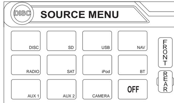
This menu allows you to select a source for the front or rear zone. Touch FRONT or REAR to choose the zone for which you would like to specify the source.
