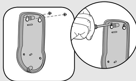
Mount Intercom with small silver screws. See mounting template on page 3. Screw the top two screws halfway into the mounting surface. Place back of intercom over screws. Tighten screws.
