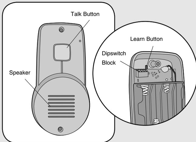
**Talk Button:** To talk, hold down the Talk button and all intercoms in the network will receive the signal. When holding down the Talk button on a different intercom, a secure channel is created and the other intercoms in the network do not hear the conversation.
