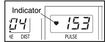
If the displayed pulse appears to be too high or too low, or if your pulse is not displayed, lift your thumb off the sensor and allow the display to reset. Press down again on the sensor as described above.
