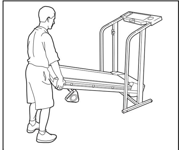
2. Move your right hand to the position shown at the right, and hold the treadmill firmly. Raise the treadmill until the storage latch locks over the frame guide. If necessary, turn the Incline leg as you raise the treadmill. **Make sure that the storage latch closes fully over the frame guide.**
