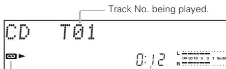
This indicator lights up when CD is loaded. Elapsed time of track being played.
