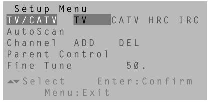
**TV/CATV SELECT:** To select TV signal input between off-air and cable service. **AutoScan:** To search for available TV /CATV channels.
