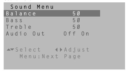
**Balance:** To adjust the left and right audio balance.
