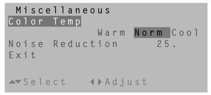
**Color Temp:** To select your color temperture between **Warm**, **Norm** and **Cool**. **Noise Reduction:** To reduce the noise of picture.
