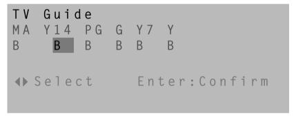
Select **TV Guide** to set rating grade. Use remote control arrow keys to move cursor to desired rating grade, and it will turn red. Press **ENTER** key to set block **(B)** or unblock **(U)** condition.
