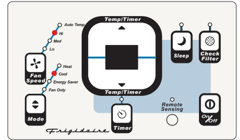
Note: This feature can be used with any combination of FAN Speeds, Timer, or Sleep Modes. When in the "Heat" Mode, the fan will run continuously while heat is needed. The temperature will automatically be maintained anywhere between 55°F (13°C) and 80°F (27°C). When the room set temperature is satisfied, the fan will cycle off and on to circulate and sample the room air.
