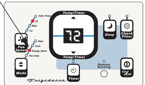
Note: In this mode, the fan will continue to run for 3 minutes after the compressor shuts off. The fan then cycles on for 2 minutes at 10 minute intervals until the room temperature is above the set temperature, at which time the unit cooling system starts again.
