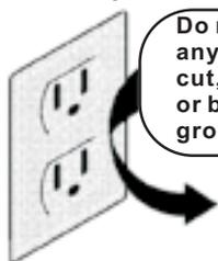
Do not, under any circumstances, cut, remove, or bypass the grounding prong.
