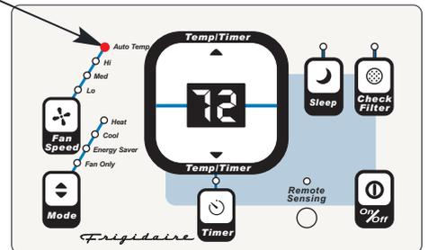
Note: The fan speed will begin in HI, then adjust to MED and LO as the room temperature conditions indicates. For example in cooling, if the room doesn't get too warm it will stay at LO. If the room temperature rises quickly, such as a door being opened, it will automatically go to HI speed. The fan speeds will adjust back to LO as the room returns to the original set temperature.
