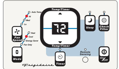
Note: Tap or hold either up(^) or down(v) button until the desired temperature is seen on display. This temperature will be automatically maintained anywhere between 60F (16°C) and 90F (32°C) for cooling mode. The Temperature will be automatically maintained anywhere between 55F (13°C) and 80F (27°C) for heating mode. If you want the display to read the actual room temperature, "FAN SEE ONLY MODE".
