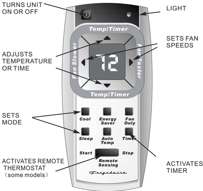
REMOTE CONTROL w/DISPLAY & REMOTE SENSING BUTTON
