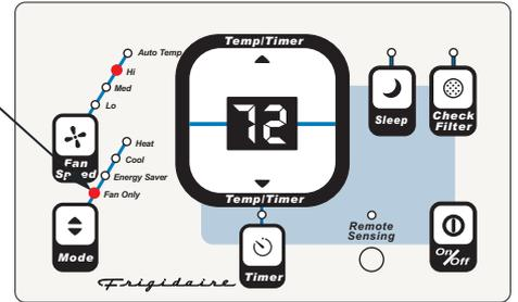
Note: Use this function only when cooling is not desired, such as for room air circulation. You can choose any fan speed you prefer, EXCEPT AUTO FAN. During this function, the display will show the actual current temperature, not the set temperature as in the cooling mode.
