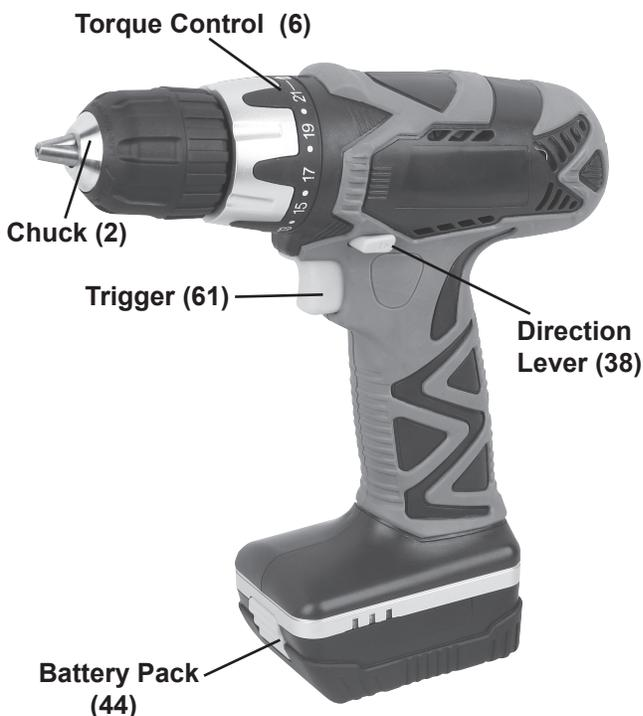
1. In order to use the included screwdriver bits, you must first attach the Bit Adapter (62) into the Chuck (2). With the Chuck pointing away from you, turn the Chuck counterclockwise. Insert the shank of the Bit Adapter all the way into the Chuck. Turn the Chuck clockwise to lock the Bit Adapter in place.
