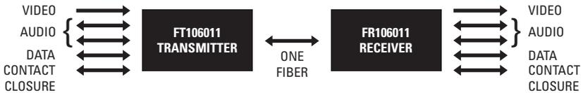
**Figure 1.** FT106011/FR106011 Video, Audio, Data, and Contact Closure Transmission
