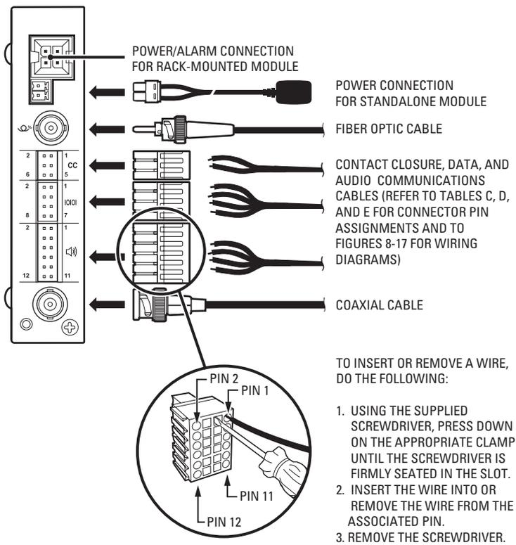
**Figure 7.** FT106011 Transmitter/FR106011 Receiver Connections
