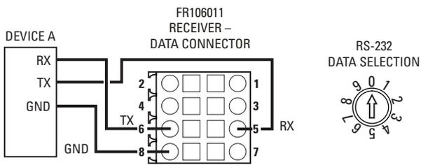
**RS-232 DATA CONNECTIONS BETWEEN DEVICE A AND FR106011 RECEIVER**
