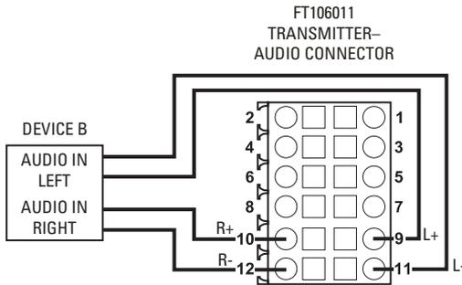
**Figure 16.** Balanced Audio Wiring
