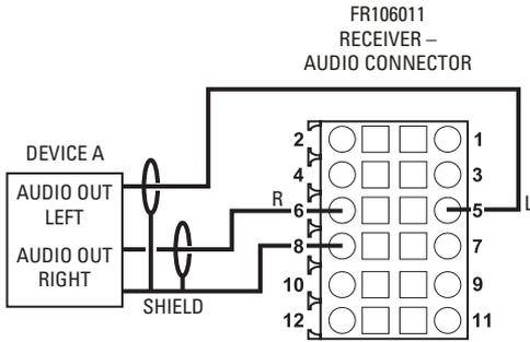
**UNBALANCED AUDIO CONNECTIONS BETWEEN DEVICE A AND FR106011 RECEIVER**
