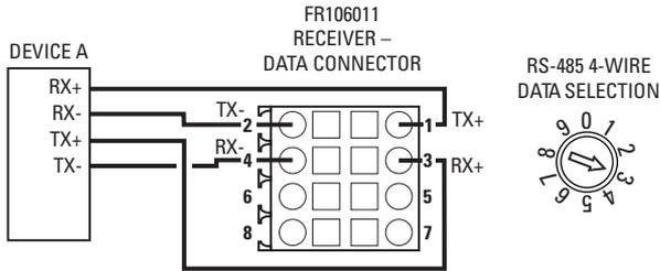
**RS-485 4-WIRE DATA CONNECTIONS BETWEEN DEVICE A AND FR106011 RECEIVER**
