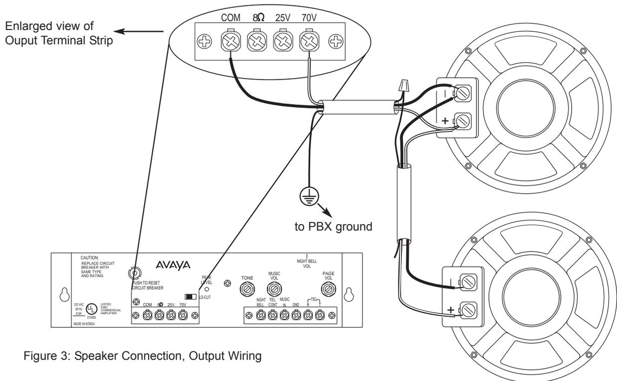
Figure 3: Speaker Connection, Output Wiring
