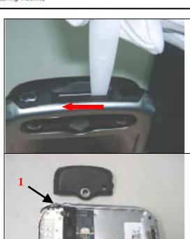
There are three hooks which fix the antenna cover and bezel.
