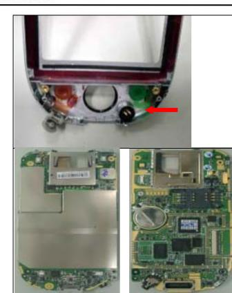
If MIC need to be replaced, just take it out from its place slightly by using tweezers.
