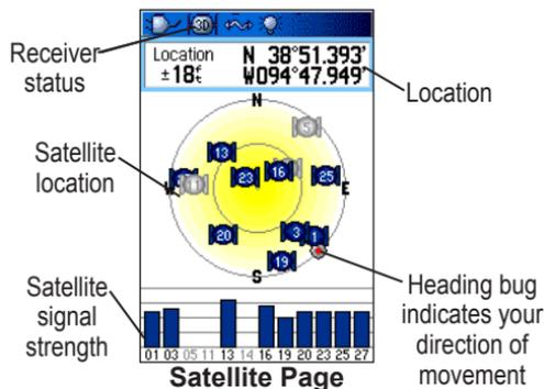
The larger circle beneath the satellite icons represents the horizon surrounding you and the smaller circle a position approximately 45° above your current position. Imagine that you are in the center of a clear dome with the satellites moving over its outer surface.
