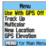
**Use With GPS Off/On**—enables you to turn the GPS receiver on or off.
