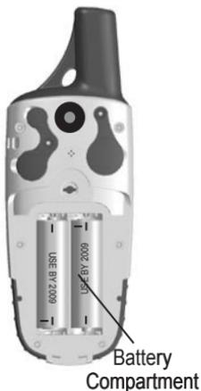
Remove the batteries from your GPSMAP 60Cx when you do not expect to use the unit for several months. Stored data is not lost when batteries are removed.
