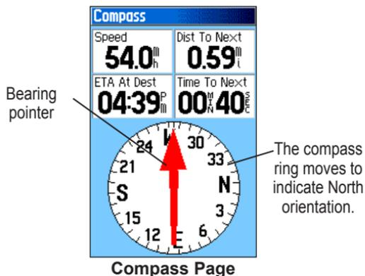
When navigating, the Compass Page provides navigation data and directions. It uses a graphic compass ring, a bearing or course pointer, and digital data fields to show information, such as current speed, distance to the next point on the route, and estimated arrival time.
