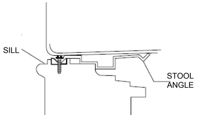
3. Fasten cabinet to window sill using two 3/4" HEX-Head screws. Pre-drill holes if needed. Add the bottom rail seal over the screws.
