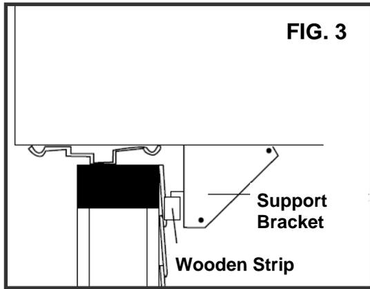
5. Screw or nail the cabinet to the wooden frame using shims if the frame is oversized, to eliminate possible noise. Remember to maintain proper slope for water elimination.
