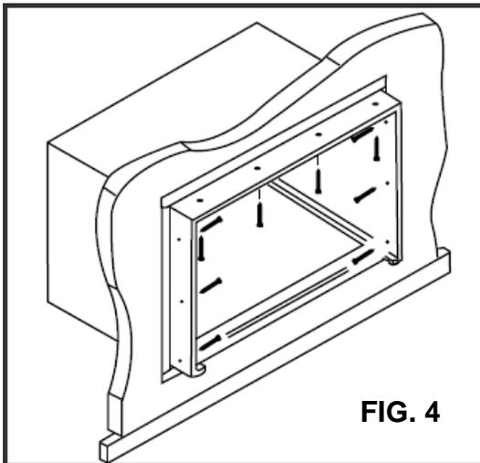
6. Install the chassis into the cabinet by following the steps described in the WINDOW MOUNTING section.
