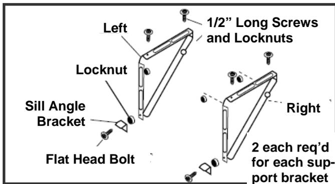
2. Assemble the sill angle brackets to the support brackets at the marked position as shown above. Hand tighten, but not all the way for any changes that may need to be made later during installation.
