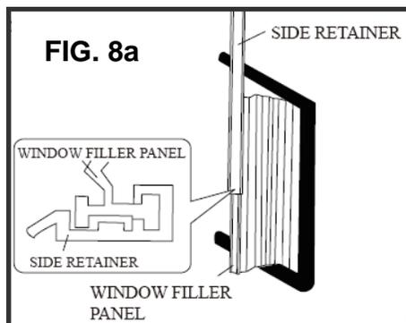
6. Insert top and bottom legs of window filler panel frame into channel in the top angle and bottom rail. Do both sides. Install side retainer to cabinet as shown. FIG 8B-9.
