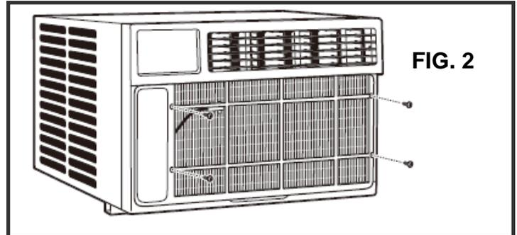
3. Locate the four faceplate screws and remove. These screws will need to be re-installed prior to mounting the air conditioner (FIG. 2 above)
