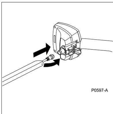
**Figure 2.6** Attaching coil cable to control box
