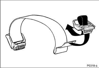
**Figure 2.11** Fitting buckle to armrest strap
