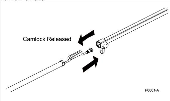
Figure 2.4 Feeding coil cable into upper shaft
