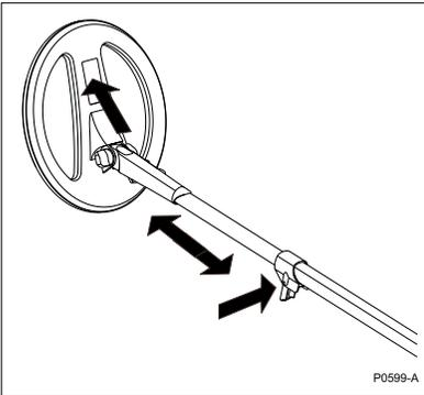
**Figure 2.9** Adjusting the shaft and angle of the search coil
