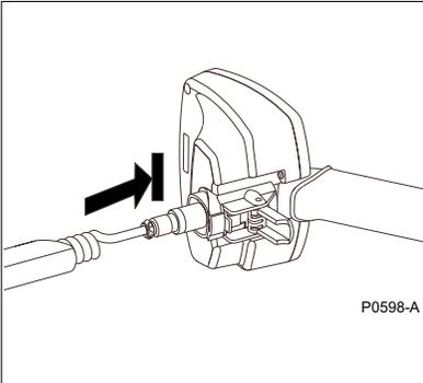
**Figure 2.8** Inserting shaft assembly into control box
