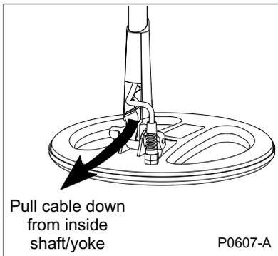
Figure 2.15 Removing cable
