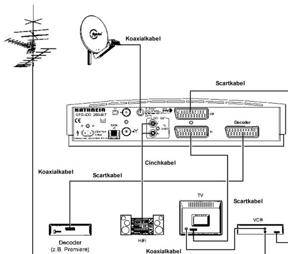
Connection of Sat receiver to TV set and video recorder with coaxial cables.
