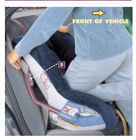
If you are using a vehicle seating location equipped with a shoulder belt, you must use only one forward-facing position locking clip on the car seat to prevent the vehicle belt system from loosening during use. With the vehicle belt system tight, fit the shoulder belt into the forward-facing position locking clip on the burgundy tube.
