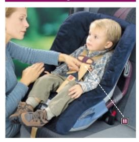
Check to be sure the shoulder straps are locked into the buckle and securing your child properly. Pull the shoulder straps up and away from your child firmly. The shoulder straps should remain locked in the buckle and should not pull more than one inch (two fingers) away from your child's chest. If the shoulder straps are too loose or unbuckle, please re-read the instructions, "Restraining Your Child", pages 58-63, and repeat steps 3-11.
