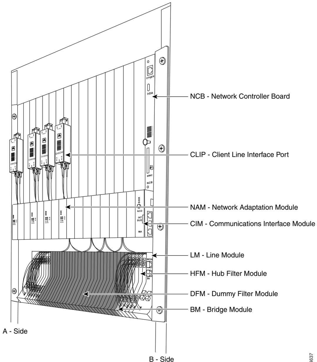
The lower portion of the ONS 15252 MCU is referred to as the passive optical shelf. The passive optical shelf has an A side and B side. The A side of the ONS 15252 MCU is located on the left side of the passive optical shelf, as seen from the front. The A-side LM contains one line IN port (FC), one line OUT port (FC), and two line-monitoring ports (SC). The line-monitoring ports make it possible to monitor the A-side incoming and outgoing DWDM optical signals.
